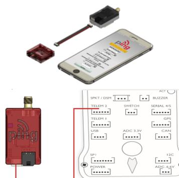
Any antenna certified to TSO-C66, TSO-C74, TSO-C112 with a peak gain of 4 dBi or less, a omni-directional radiation pattern, and a VSWR of 1.8 or less at 1090MHz is approved for use with this device and will ensure conformance to all applicable standards for RF emissions.
