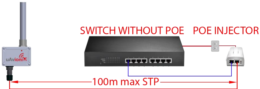
pingStation install with POE injector
