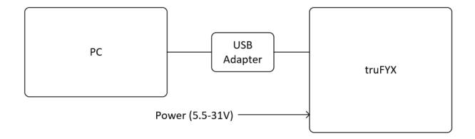
Launch uCenter and connect to the receiver on the COM port which matches the serial port assigned to the USB adapter. Set the Baudrate to 115200 bps.
