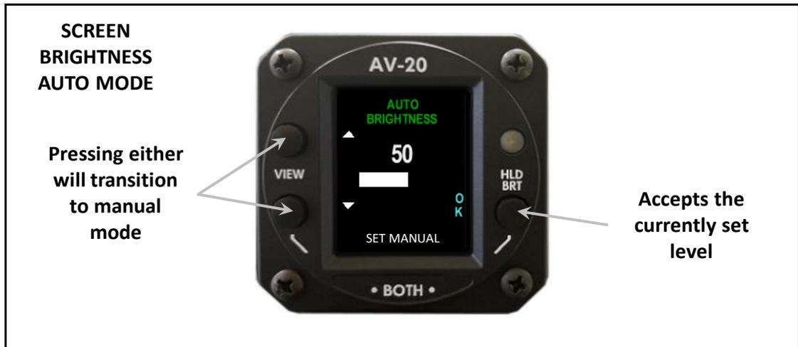
When in manual mode, pressing the up or down arrows will adjust the screen brightness. Pressing the right button will accept the value. Pressing ●BOTH● will return to auto mode.
