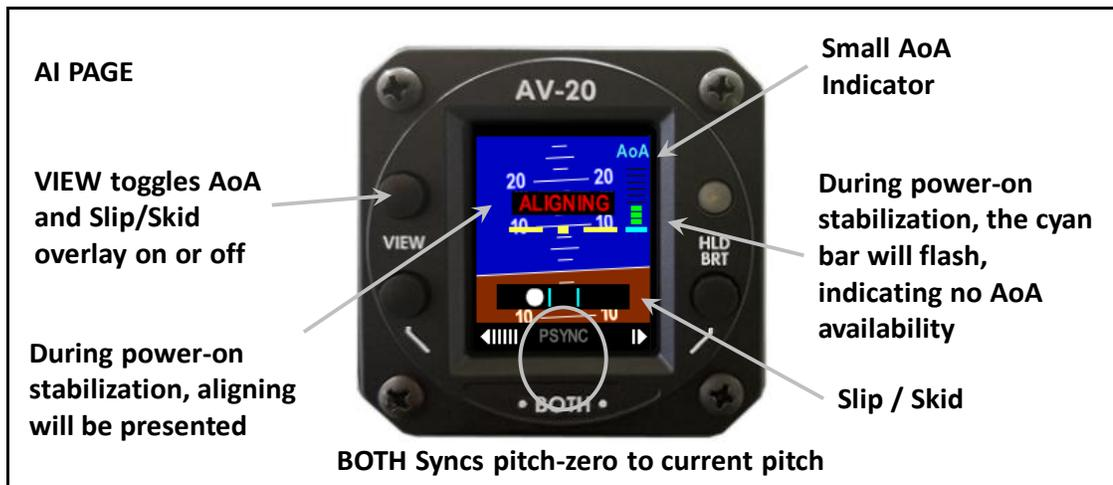
This display can be configured to automatically pop up when power is lost during flight.
