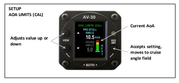
• The upper limit (pre-stall angle) is configured to coincide with the onset of the aircraft's existing stall warning system and is typically on the order of 10 to 15 degrees. This limit is set with the aircraft in its "base-to-final" configuration with flaps and gear set to their normal positions for this
