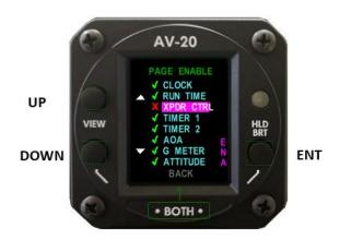
In the PAGE ENABLE sub menu of SETUP, activate the XPDR CTRL page by pressing ENA. A green check mark indicates enabled and a red X indicates disabled.
