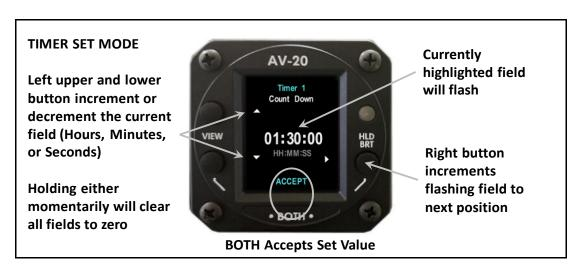
Once the set value is accepted, this value is loaded into both the upper (active) and lower (Set Value) fields on the timer page.
