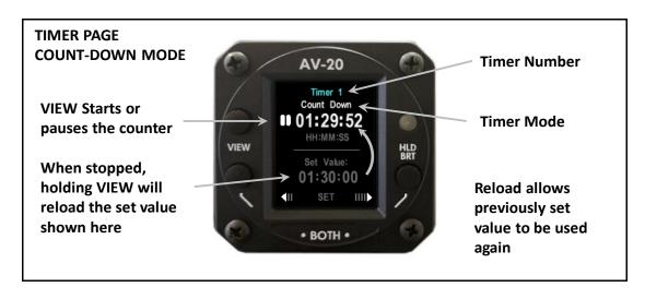
Once the timer is started and the value runs down to zero, a timer alert will be generated.
