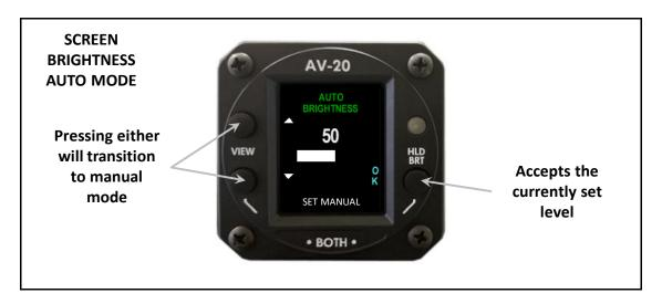
When in manual mode, pressing the up or down arrows will adjust the screen brightness. Pressing the right button will accept the value. Pressing ●BOTH● will return to auto mode.
