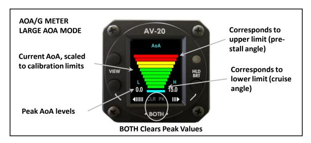
During power-on stabilization, the cyan lower bar will blink and a red X will cover the AoA label, indicating that no valid AoA can be determined. This applies to all color-coded AoA indications provided on different pages.
