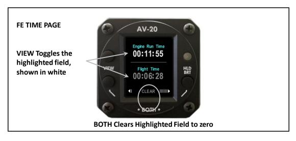
Either timer can be independently set to zero by selecting it and clearing the value.
