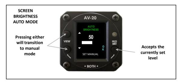
When in manual mode, pressing the up or down arrows will adjust the screen brightness. Pressing the right button will accept the value. Pressing ●BOTH● will revert to auto mode.
