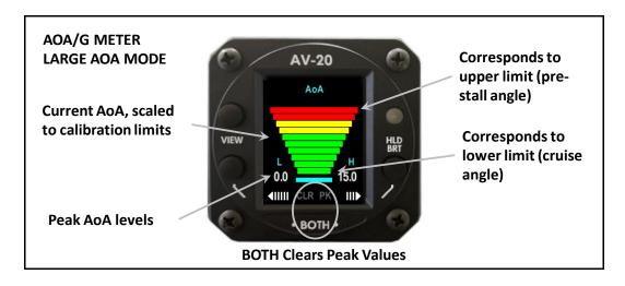
During power-on stabilization, the cyan lower bar will blink and a red X will cover the AoA label, indicating that no valid AoA can be determined. This applies to all color-coded AoA indications provided on different pages.
