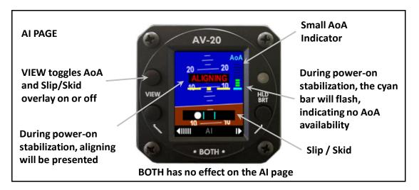
This display can be configured to automatically pop up when power is lost during flight.
