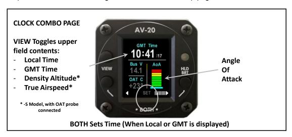
•BOTH• enters the clock set function when either the local time or GMT time is being displayed in the upper field. The set mode allows the current GMT time to be set, along with a local time offset. If time has been lost due to failure of the internal keep-alive battery, the time will flash.
