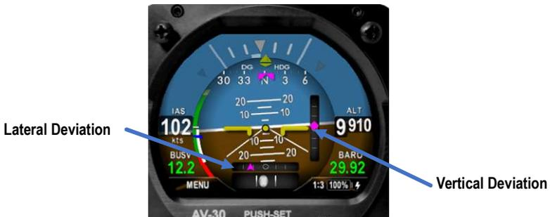
There are three independently customizable pages which are selected round-robin fashion by sequentially pressing the Page Selection button (shown as page 1 of 3 in the figures above). Each page can be configured to show various supplemental parameters as overlays.
