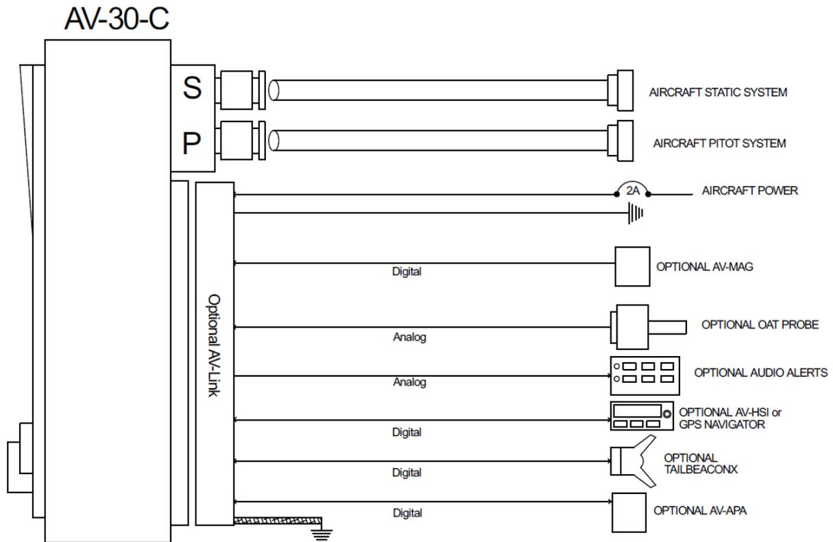
Figure 3: AV-30-C Aircraft Systems Interfaces – AI Mode
