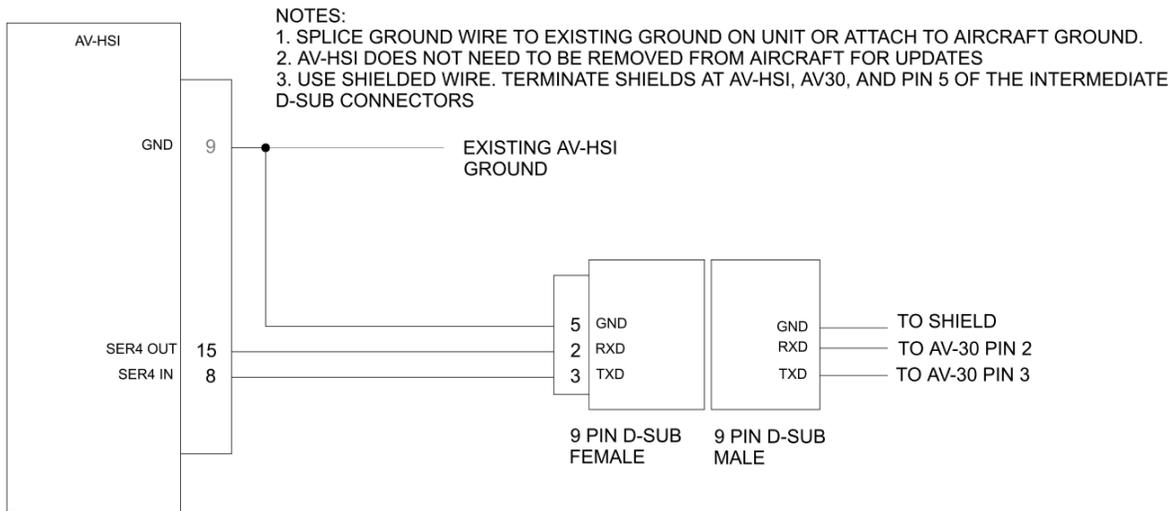
Figure 79: AV-HSI Update With AV-30-C Using Serial 4
