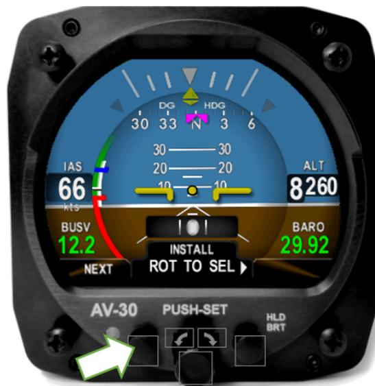
Figure 95: Install Mode Selection
