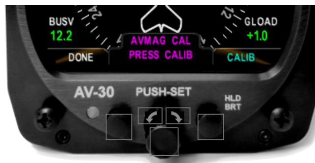
Figure 53: AV-Mag Calibration Entry
