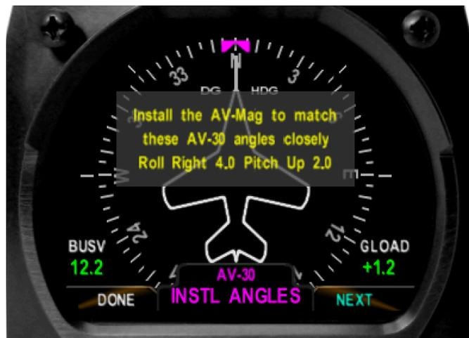
Adjust the AV-Mag mounting attitude to match that of the AV-30-C as closely as possible. Simultaneously, the AV-Mag should be oriented as parallel to the line of flight as possible.
