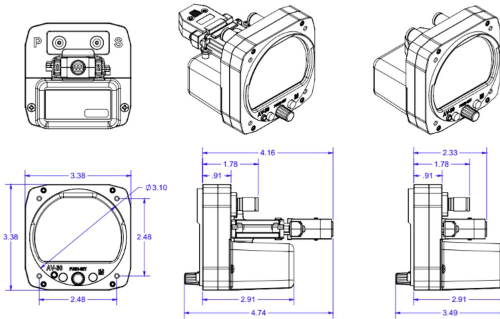
Figure 6: Mechanical Drawing with Extended NiMH Battery
