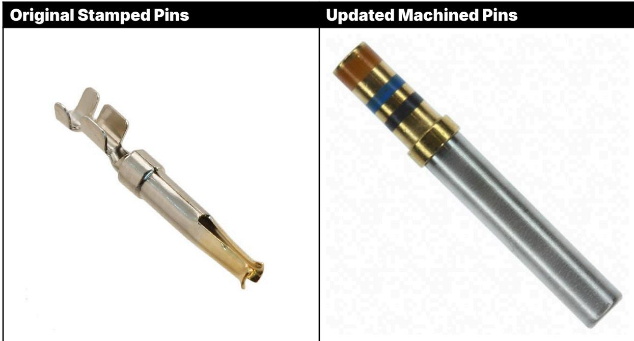
If your kit includes machined pins, a Daniels AFM8 crimp tool using a K13-1 positioner or equivalent M22520/2-01 tool should be used. If your installation kit includes the original stamped pins, a NorComp 180-701-170-000 hand crimper or equivalent should be used.
