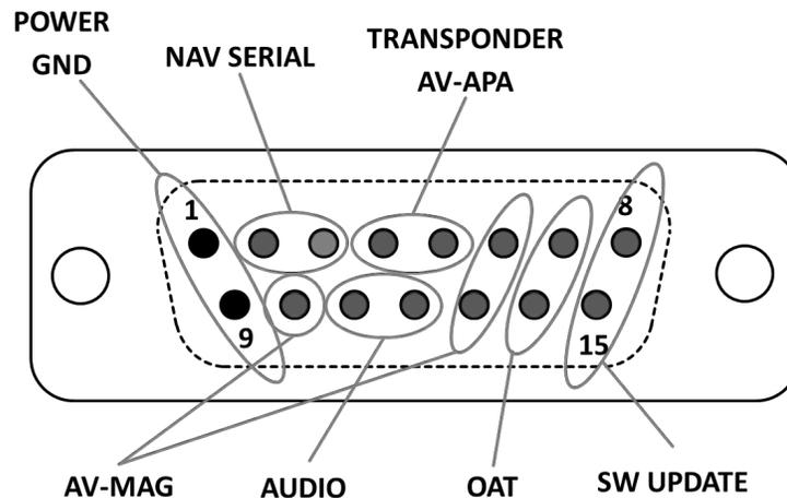
Figure 17: Unit Connections - DB-15, Male (Rear Unit View)
