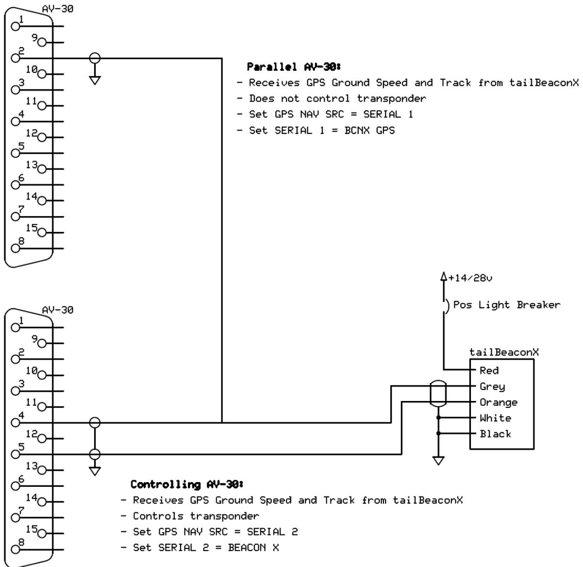
Figure 36: Parallel tailBeaconX or echoESX GPS Connections
