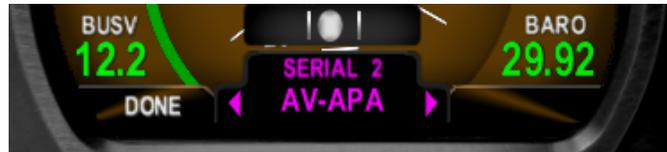
Navigate to AV-APA configuration option (AV-APA CFG) and select the appropriate autopilot that will be connected.
