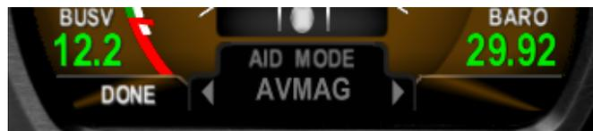
Enter the AV-30-C installation menu again and navigate to the AV-Mag installation menu (AVMAG INSTL). Push the center rotary knob, then press the right button to begin the installation process. If AV-Mag is not properly connected, the version will indicate 'Not detected'.
