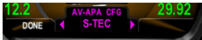
If connecting a device to the AV-APA pass-through port, navigate to the AV-APA passthrough option (AV-APA THRU) and select the appropriate device that is connected.
