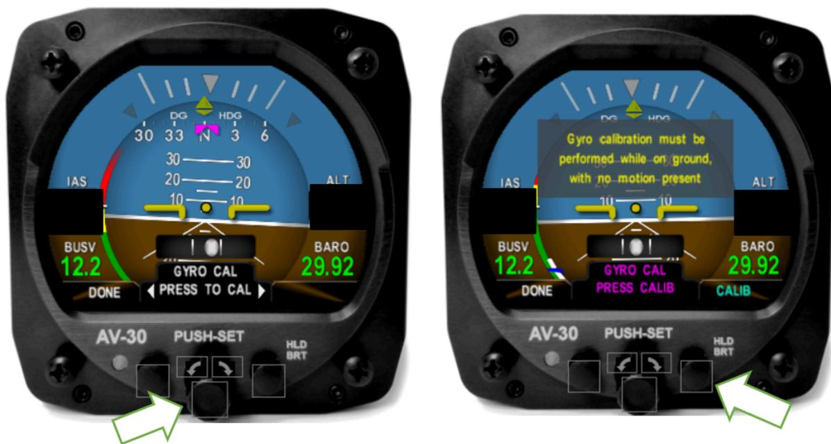
Figure 96: Gyro Calibration Selection
