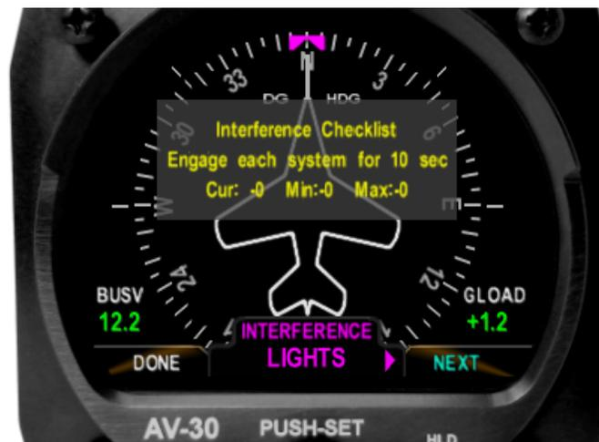
Use the rotary knob to step through each system in the checklist and monitor the magnetic field deviation value.
