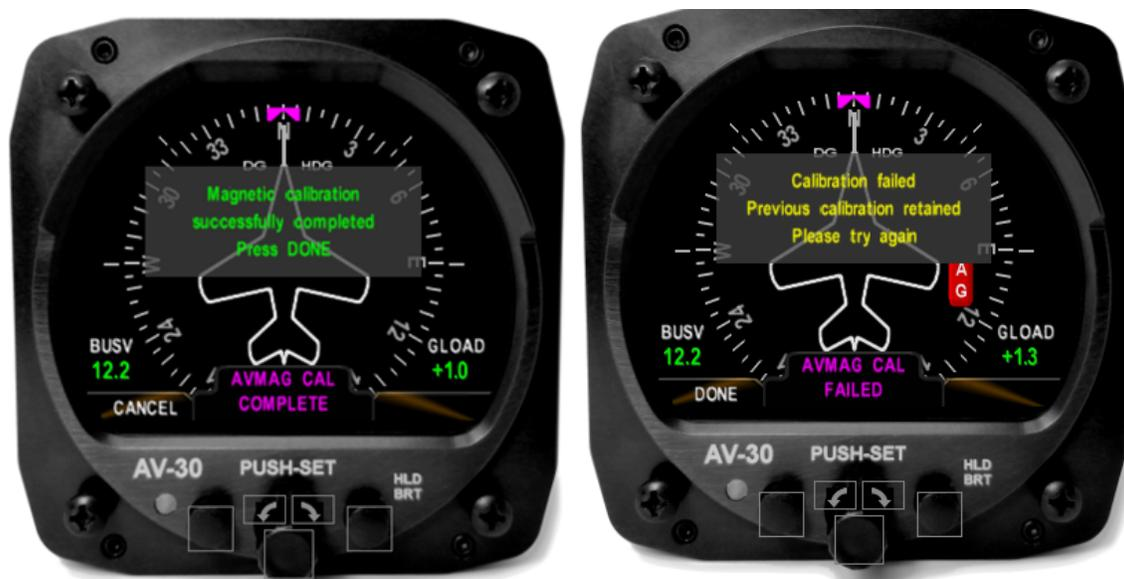
Figure 57: AVMAG CAL Success and Failure Screens
