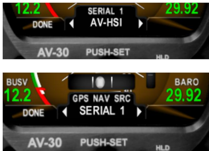
Configuration of the AV-HSI is performed through the AV-30-C Installation Menu, under the heading AVHSI CFG. This menu appears in white and is selectable if the AV-30-C detects a connected AV-HSI. Select by pressing the center knob.
