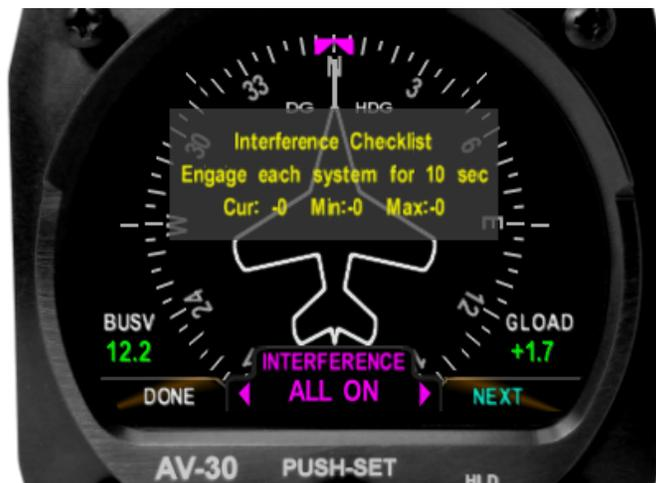
The deviation value indicates the magnitude and direction of the magnetic reading with respect to the Earth's magnetic field. A relatively small deviation near zero indicates little or no magnetic field interference, while a larger negative or positive deviation indicates the AV-Mag is sensing magnetic fields in addition to the Earth's. These additional fields must be minimized in order for the AV-Mag to be accurate.
