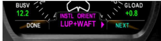
The AV-Mag uses an internal sensor to detect which orientations are possible and indicates them on screen. The selected orientation should be one of those self-detected options.
