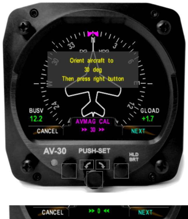
Figure 56: AVMAG CAL Orientation Guide
