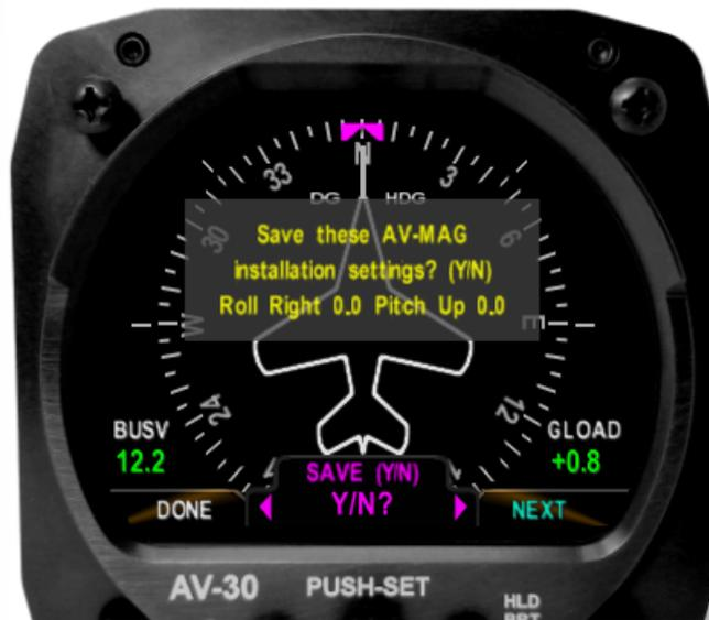
After angles have been saved, calibration may begin. Record the installation selections and parameters in Table 51.
