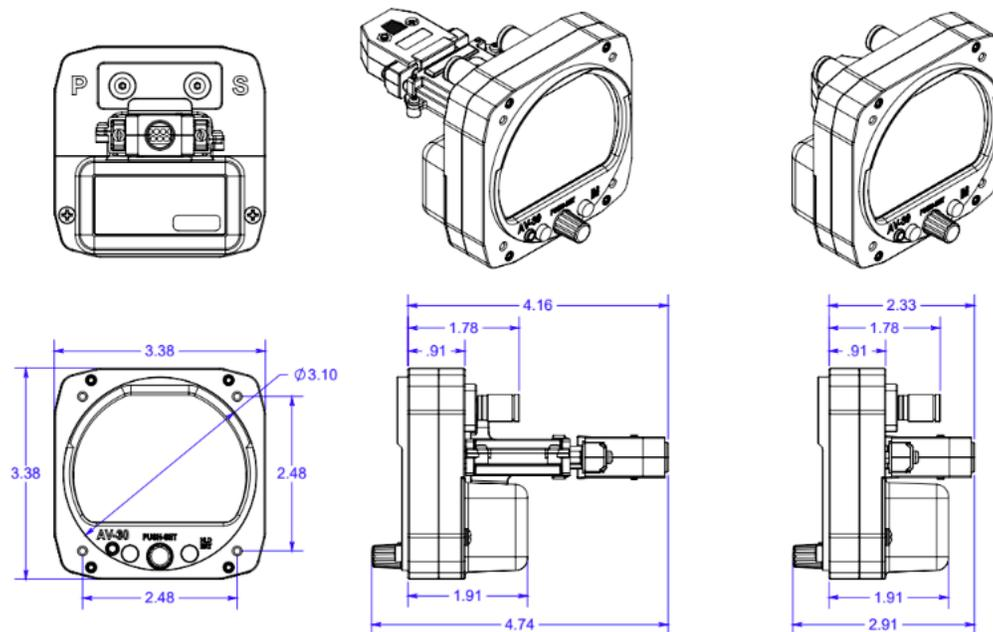
Figure 5: Mechanical Drawing with Standard Li-Ion Battery
