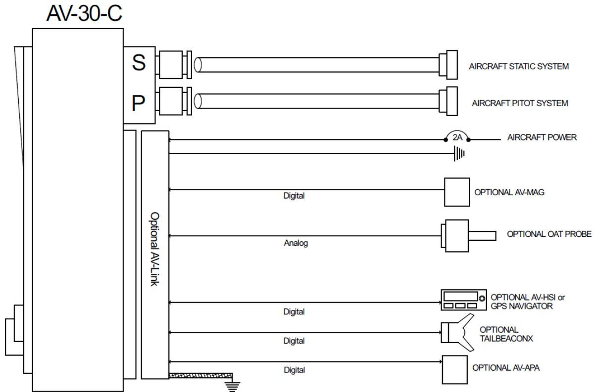
Figure 4: AV-30-C Aircraft Systems Interfaces – DG Mode
