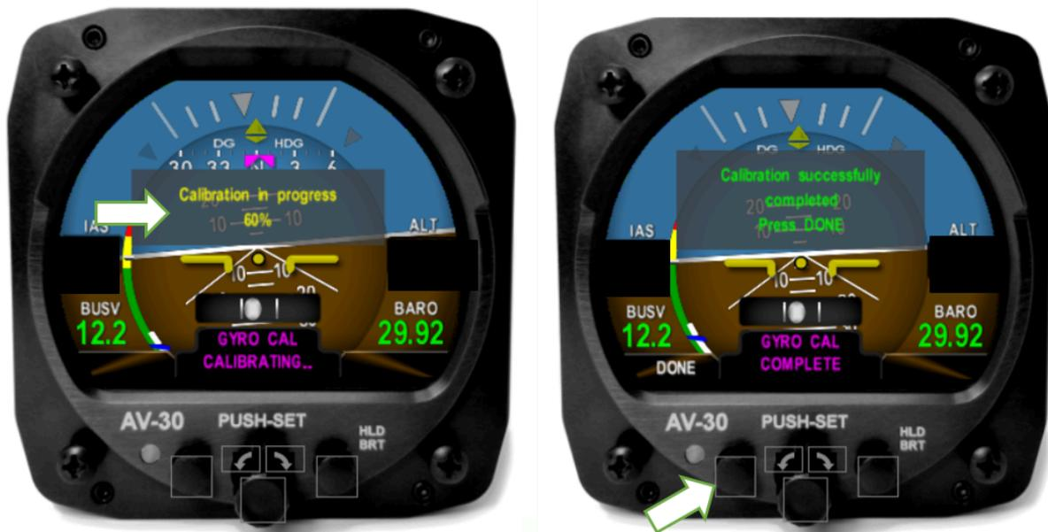
Figure 97: Gyro Calibration Procedure
