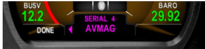
While SERIAL 4 is set to AVMAG, the AHRS aiding mode (AID MODE) will automatically be set to AVMAG and cannot be changed.
