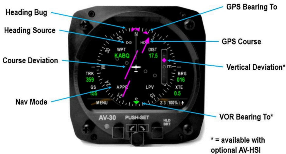
Figure 35: Non-Slaved DG HSI User Interface
