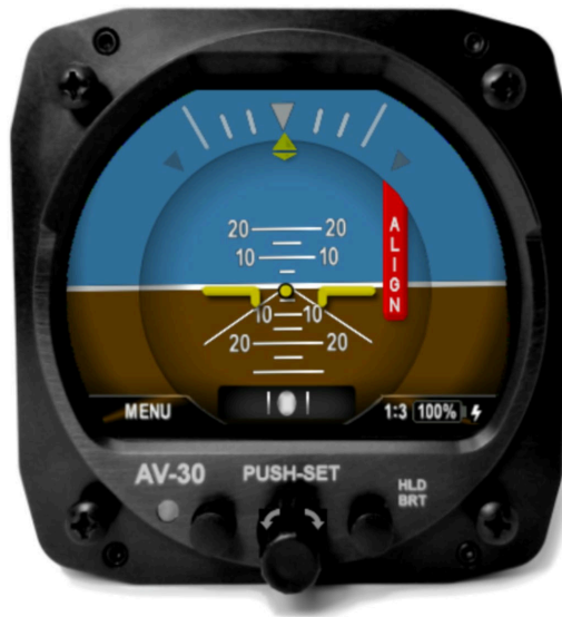
Figure 16: AI Mode, Attitude Indicator
