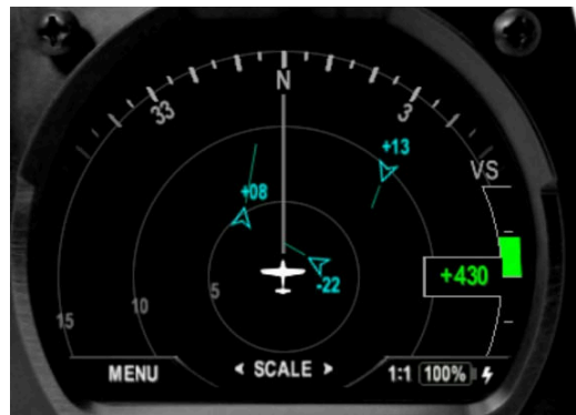
Figure 50: MFD with VSI Overlay
