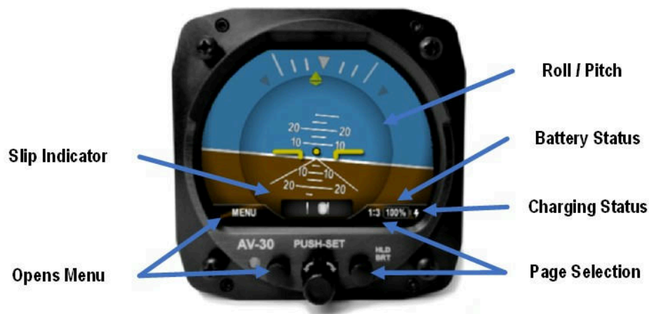
Figure 13: Basic AI Mode User Interface
