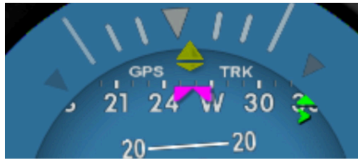
Figure 21: AI Mode, Direction Indication, Bearing To Off-Screen
