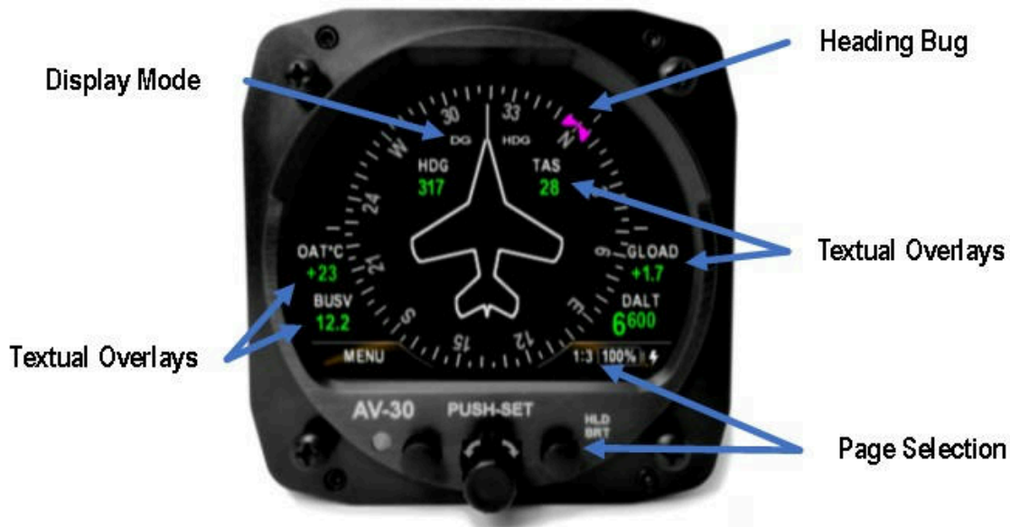
Figure 34: Basic DG Rose Mode User Interface
