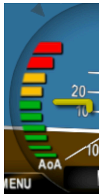
Figure 23: AI Mode, AoA Indication
