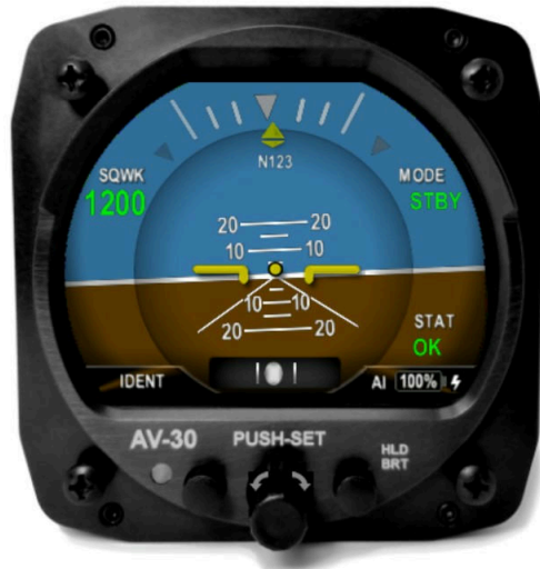
Figure 54: Reversionary Attitude Indicator
