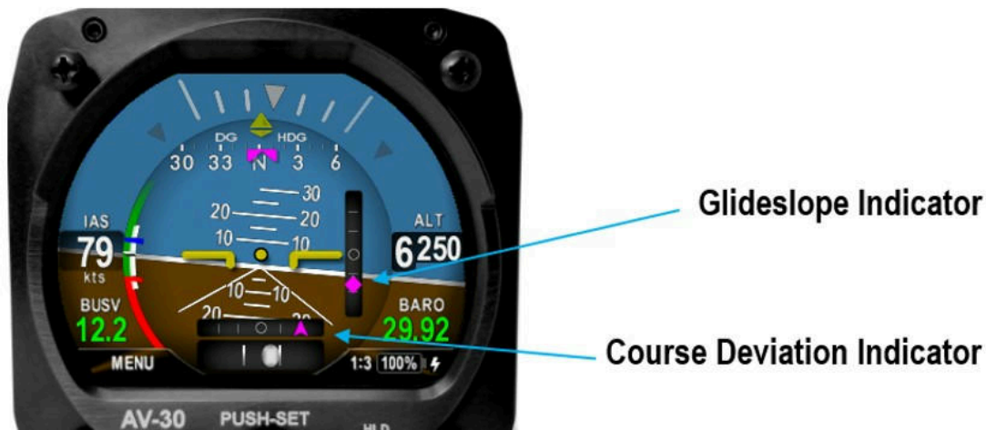
Figure 27: AI Mode, Course Deviation and Glideslope Indication
