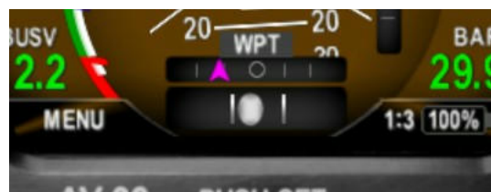
Figure 30: AI Mode, Waypoint Indication
