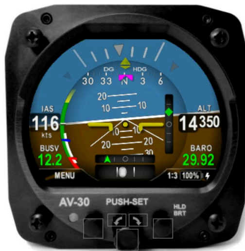
Figure 28: AI Mode, ILS Course Deviation and Glideslope Indication
