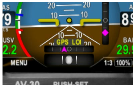
Figure 29: AI Mode, GPS LOI Indication
