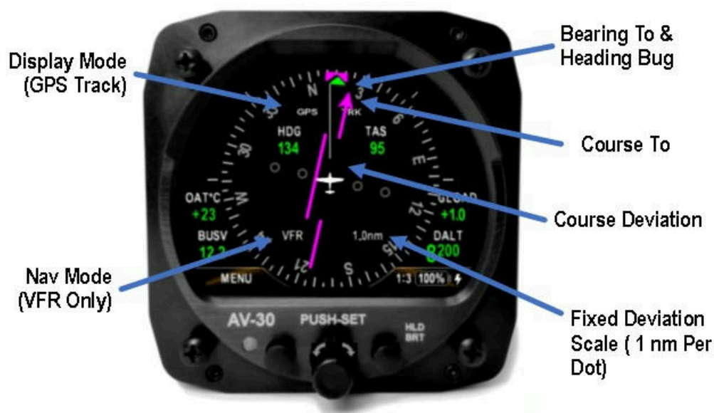
Figure 37: GPS-Slaved HSI Mode with VFR GPS
