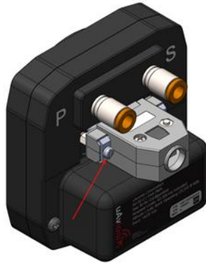
Figure 19 – AV-Link Backshell Connector Removal
