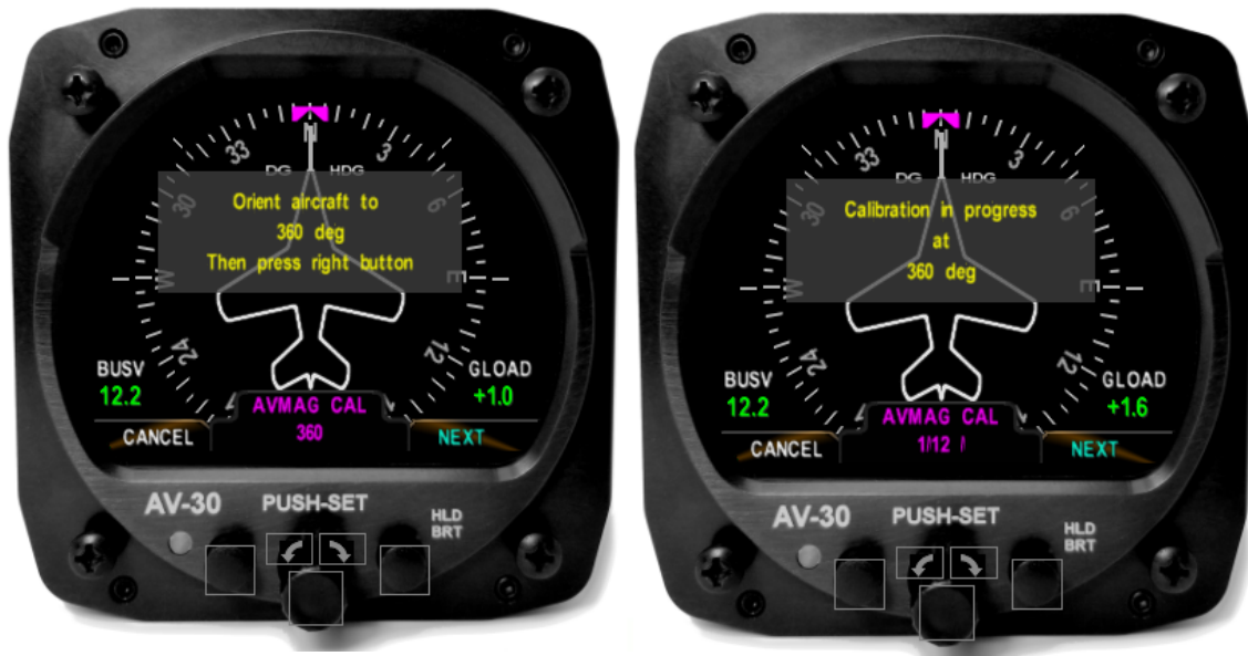
Figure 54: AVMAG CAL In-Progress
