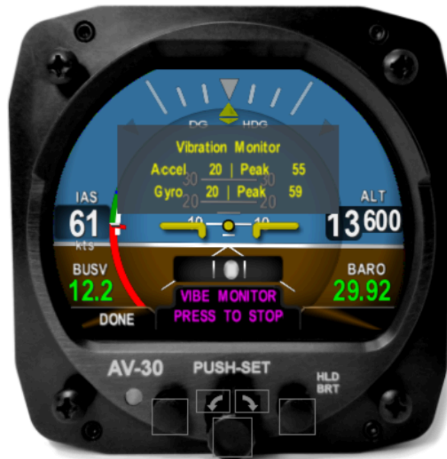
Figure 110: Vibe Monitor Operation
