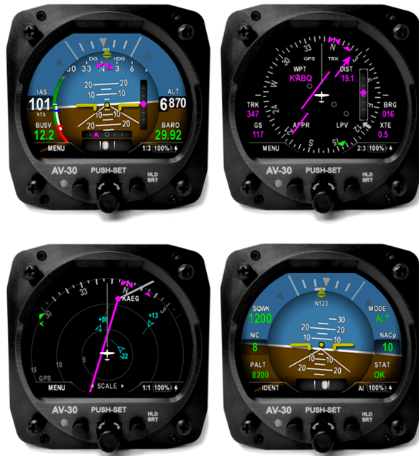
Figure 1: AV-30-E Multi Mode AI/DG/Transponder - Basic Display
