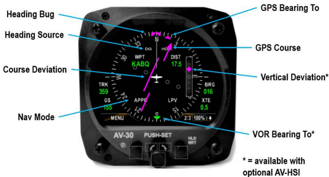
Figure 37: Non-Slaved DG HSI User Interface
