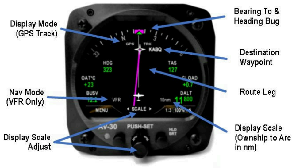
Figure 42: GPS ARC Mode
