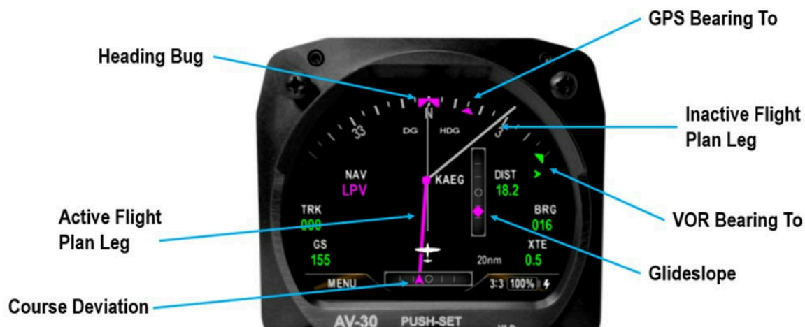
Figure 40: Arc Mode with Course Deviation and Glideslope
