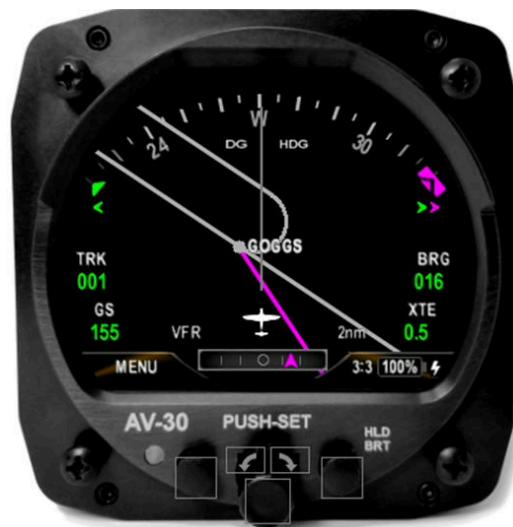
Figure 41: Arc Mode with Holding Pattern
