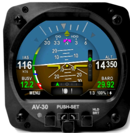
Figure 30: AI Mode, ILS Course Deviation and Glideslope Indication
