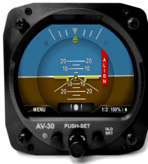
Figure 16: AI Mode, Attitude Indicator
