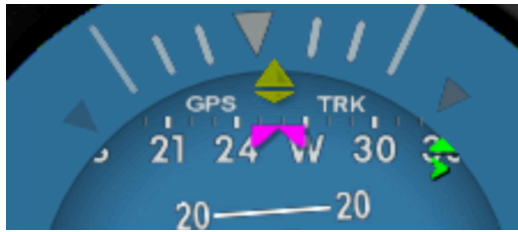
Figure 21: AI Mode, Direction Indication, Bearing To Off-Screen
