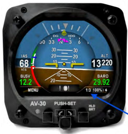
Figure 7: Page 1 of 3 showing Air Data and DG Heading
