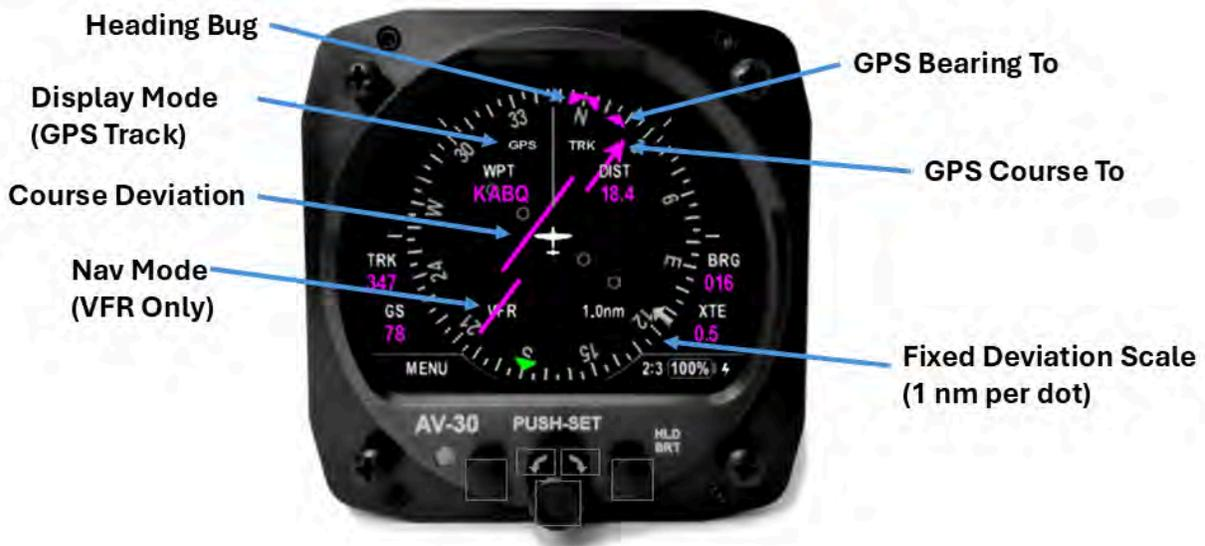
Figure 42: GPS Track HSI Mode with VFR GPS
