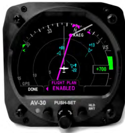
Figure 55: Flight Plan on MFD
