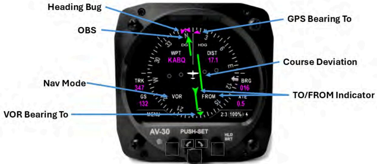
Figure 41: DG Heading HSI User Interface with VOR Guidance
