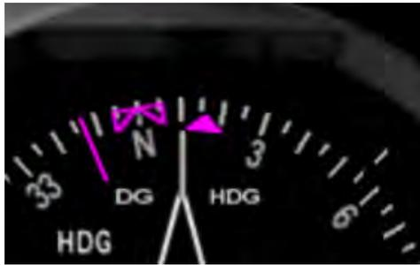
Figure 78: GPS Track Indicator on DG Heading Rose
