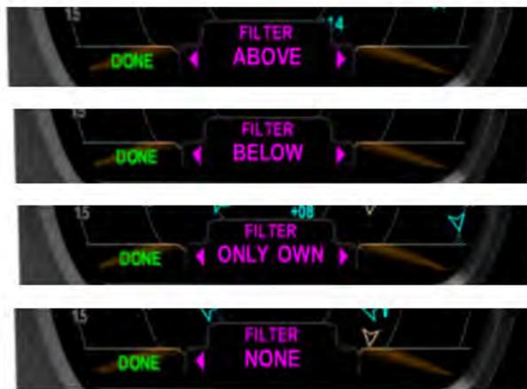
Figure 53: Examples of Alternate Filter Values
