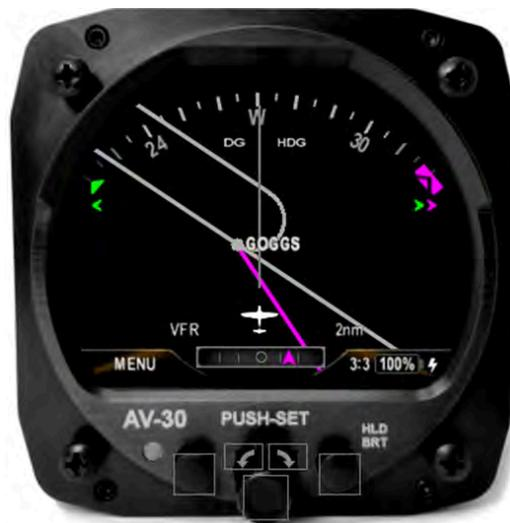
Figure 44: Arc Mode with Holding Pattern
