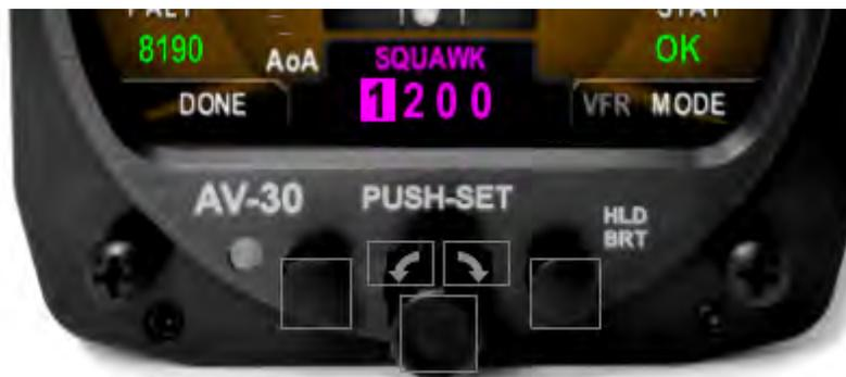
1. With 'MODE' highlighted, a single press and release of the right button will cycle through each mode selection (STBY, ON, ALT).
