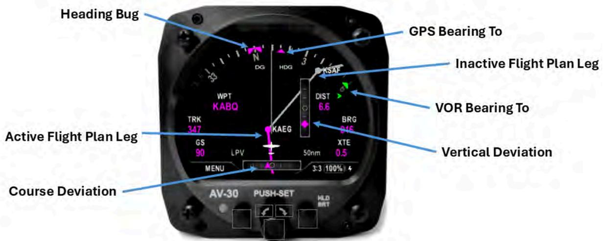
Figure 43: Arc Mode with Course Deviation and Glideslope
