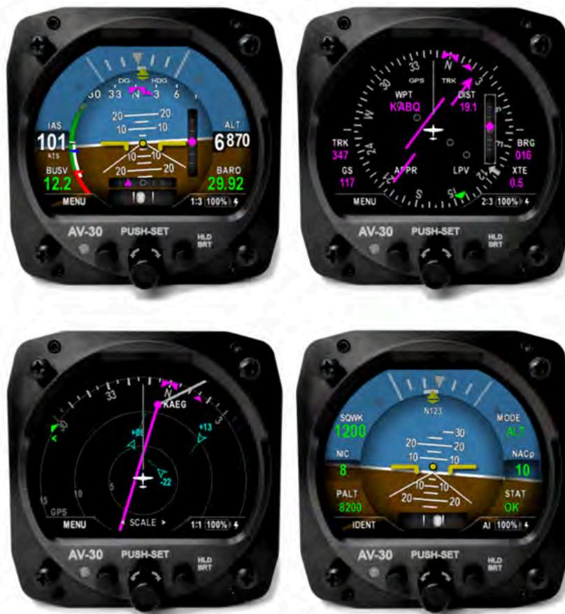
Figure 1: AV-30-E Multi Mode AI/DG/Transponder - Basic Display
