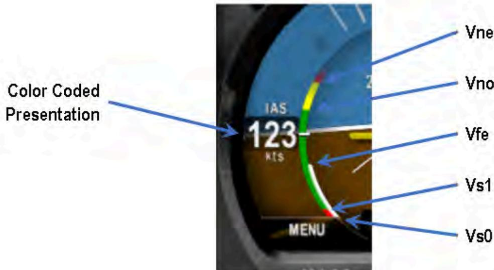
Figure 20: AI Mode, V-Speed Limits
