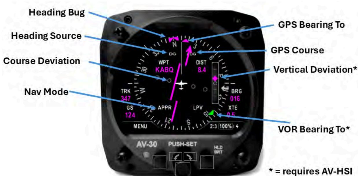
Figure 40: DG Heading HSI User Interface
