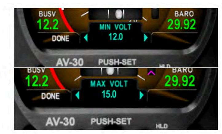
Figure 47: BUSV Threshold Setup
