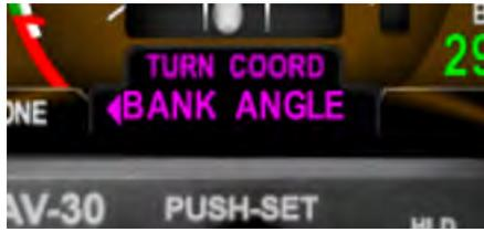
The Rate of Turn indicator consists of a flag that grows left or right from the Roll indicator. Alignment with the extended 30 degree roll mark indicates a 2-minute standard rate turn.
