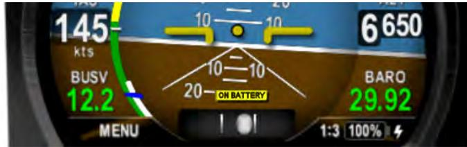
Figure 67: On Battery Operation
