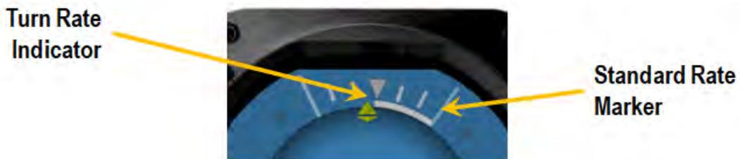
Figure 17: AI Mode, Rate of Turn Indicator
