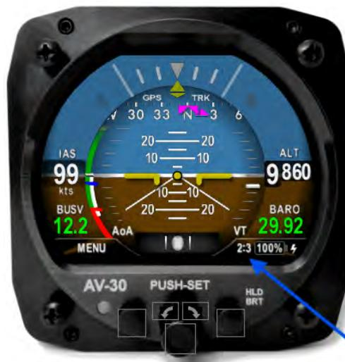
Figure 8: Page 2 of 3 showing GPS Ground Track, AoA, and Vertical Trend
