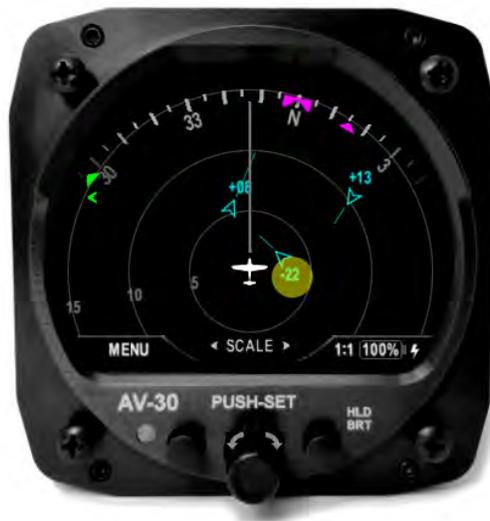
Figure 50: Traffic Target Relative Altitude
