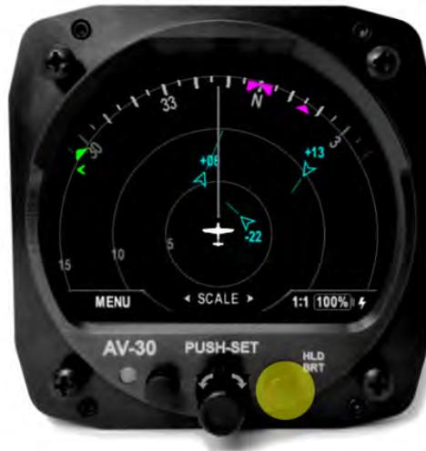
Figure 52: Traffic Reversionary AI Activation
