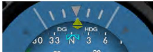
Figure 22: DG Heading with Cyan Hollow Bowtie for Autopilot
