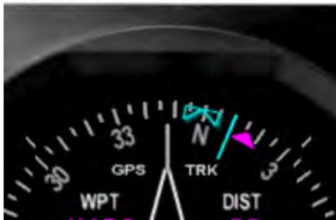
Figure 77: DG Heading Indicator on GPS Track Rose
