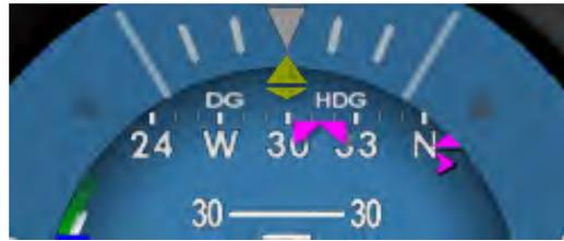
Figure 21: Solid Magenta Bowtie for General Heading Bug, Bearing To Off-Screen
