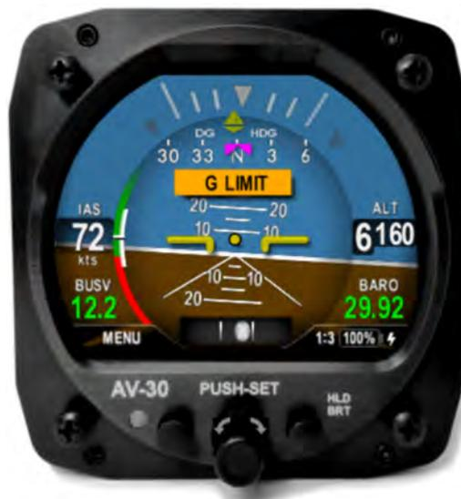
Figure 65: Example of Alert Annunciator on Screen
