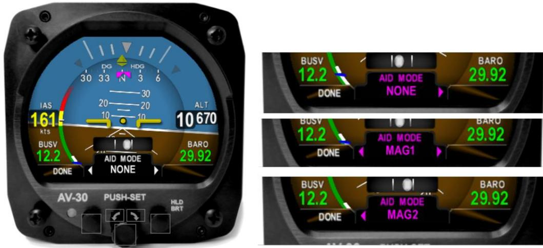
The factory setting for non-magnetometer equipped units is NONE, and the factory setting for magnetometer equipped units is MAG1. Leave the AID Mode set to the default, unless otherwise directed by uAvionix Support.
