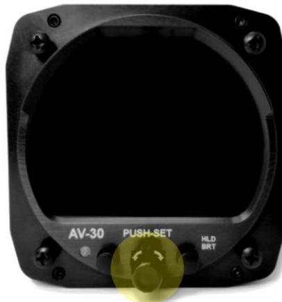
2. Push and release the left button under the MENU until the “INSTALL / ROT TO SEL” appears.
