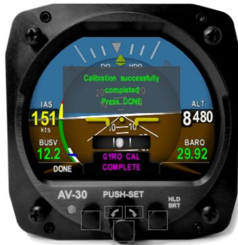
AV-30-E will indicate "Calibration successfully completed Press DONE".
