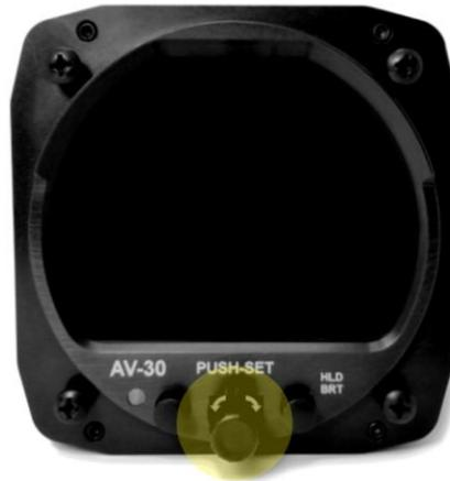
2. Keep the knob pushed until the startup screen displays, and then release.
