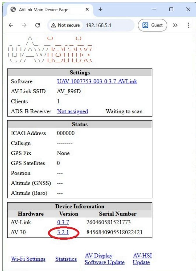
The screenshot shows the AVLink Main Device Page in a web browser. The browser address bar displays "192.168.5.1" and "Not secure". The page content includes a settings section, a status section, and a device information table. The device information table has a red circle around the version number "3.2.1" for the AV-30 hardware.
