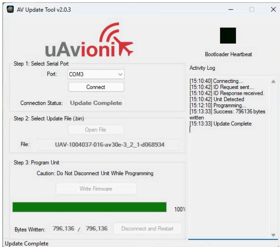
11. The unit will automatically restart. Upon restart of the unit, verify the startup screen indicates the updated software version.
