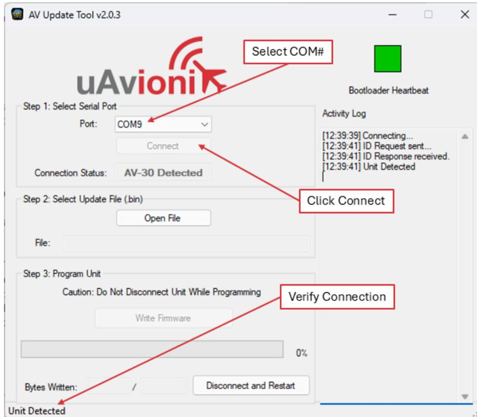
5. Proper connection has been made when the message "Unit Detected" has appeared on the bottom left corner of the AV Updater Tool. The screen on the AV-30-E will go black for the remainder of this procedure.
