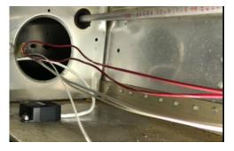
Mounting of the AV-Mag too close to wire bundles especially of high voltage or motors. Try to mount AV-Mag 18-36 inches if possible, from wire bundles or until the interference is within range.
