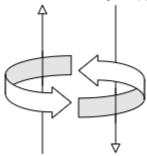
Loop or coil of wire: A loop or coil of wire concentrates the magnetic field when compared to a straight wire carrying the same current. Be mindful to avoid placing the AV-Mag in the middle of even a large loop of wire.
