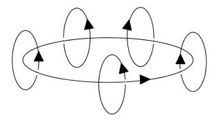
Power and ground from lights that are not tied together. This can cause a magnetic field.
