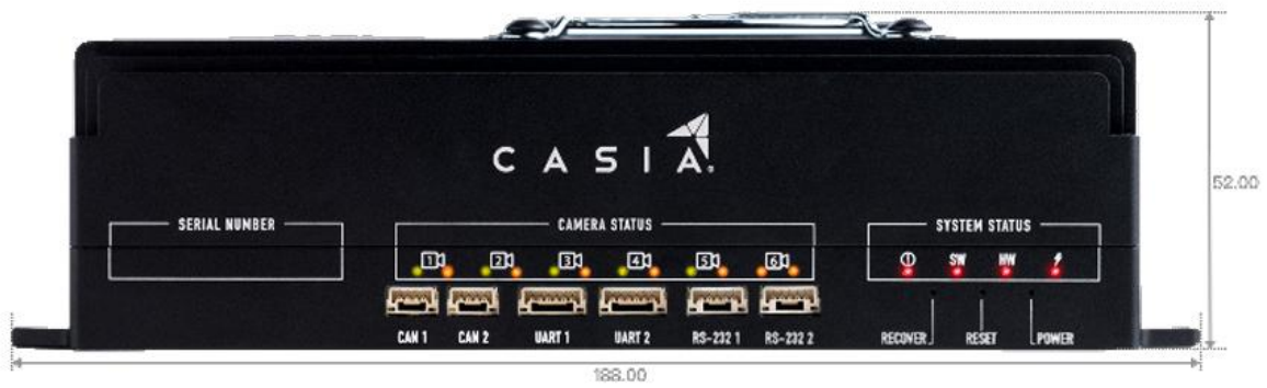
Figure 4: Casia X Front Profile with Height Dimensions
