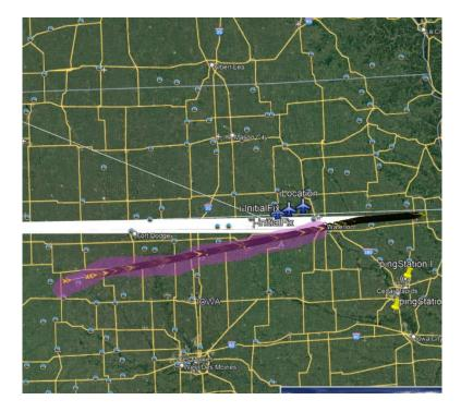
2. Then an erroneous lat/long CPR odd pairing arrived from the target aircraft (highlighted yellow below).
