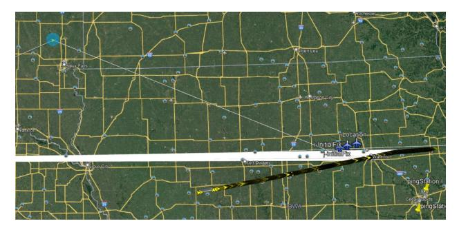
4. Subsequently received CPR data was valid and track resumed on the correct heading but offset to the west in the adjacent longitudinal zone. Refer to orange highlight below.
