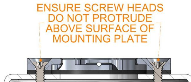
Note: Installation of the tailBeacon must be in accordance with AC 43.13-2B, Chapter 1.
