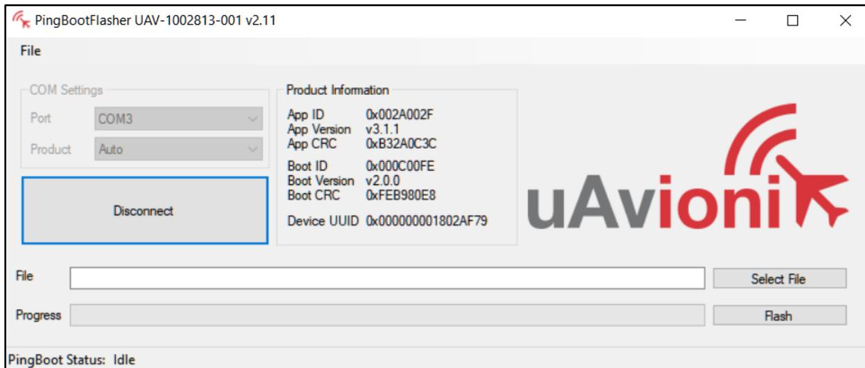
8. From the pingBootFlasher main page, press “Select File” and load the UAV file listed in Table 5-1.
