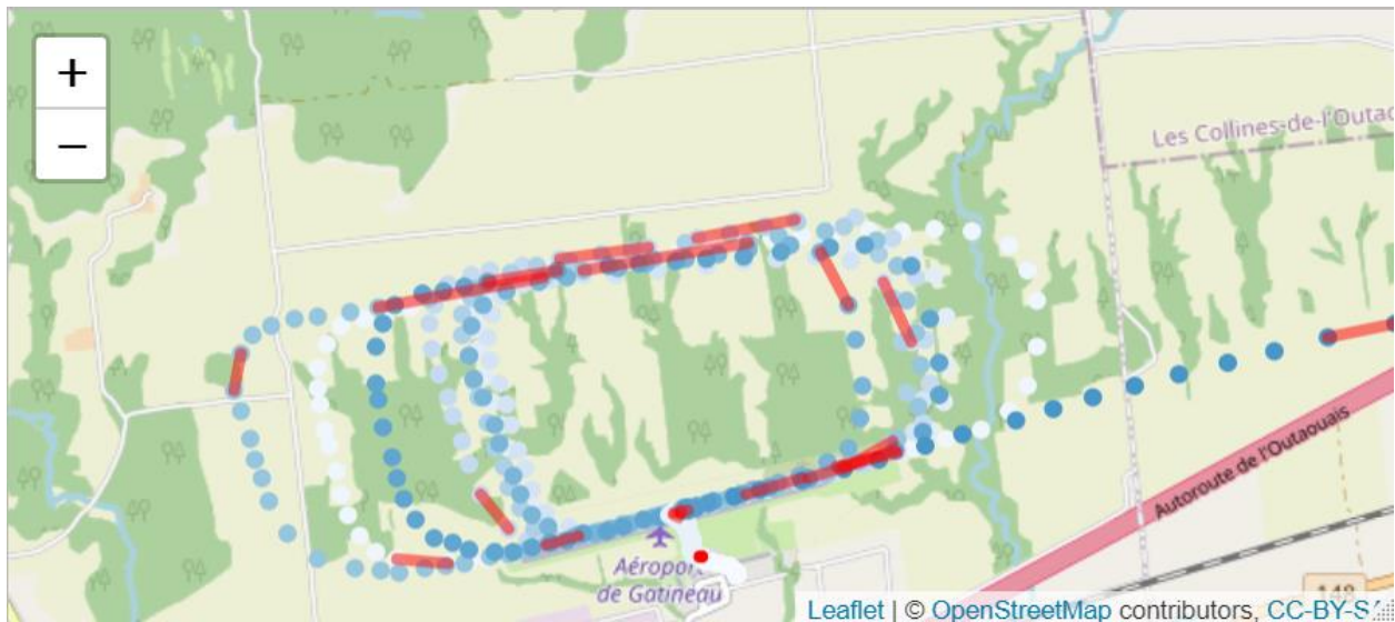
Figure 5: Example of Touch and Go Maneuvers as Observed by Aireon. Red portions are a failure of PUI of 8 seconds
