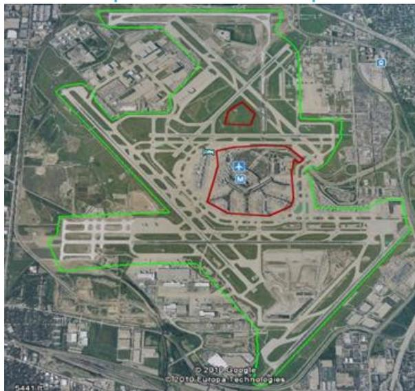
VTU-20 uses FAA approved Squitter Transmit Maps to automatically enable and disable transmission based on its location on the airfield.
