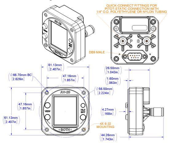
Figure 1 - Mechanical Drawing
