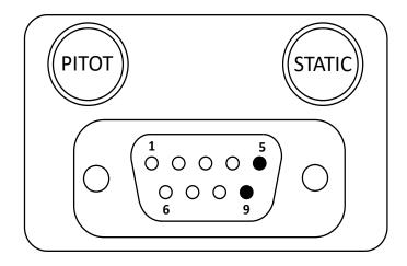
Figure 3 – Unit Connections – DB-9, Male Connector – Rear View
