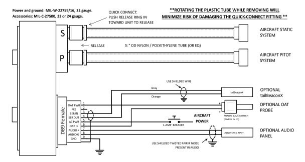
Figure 2 - Wiring Diagram
