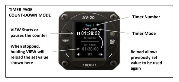
Once the timer is started and the value runs down to zero, a timer alert will be generated.
