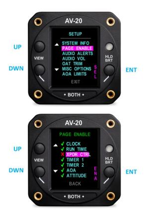
In the PAGE ENABLE sub menu of SETUP, activate the XPDR CTRL page by pressing ENA. A green check mark indicates enabled and a red X indicates disabled.
