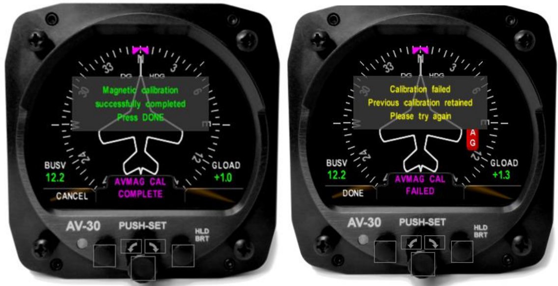
Figure 31 – AVMAG CAL Success and Failure Screens
