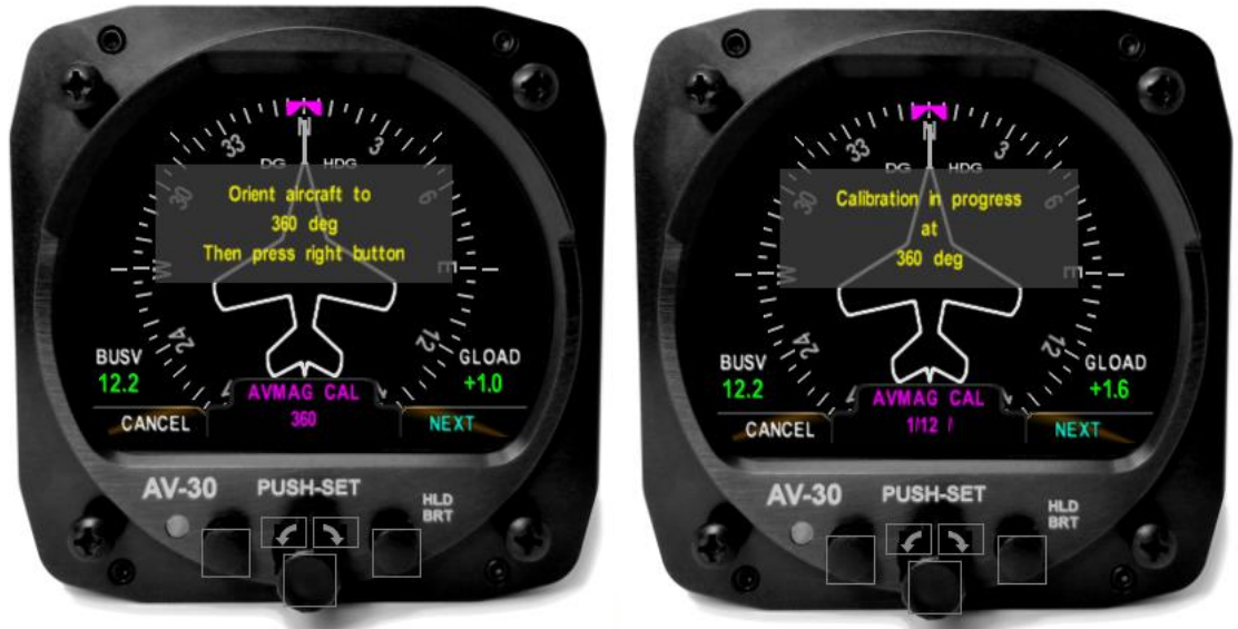
Figure 40 – AVMAG CAL In-Progress
