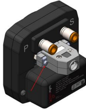
Figure 19 - AV-Link Backshell Connector Removal
