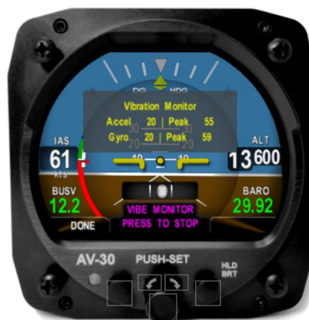
Figure 46 - Vibe Monitor Operation
