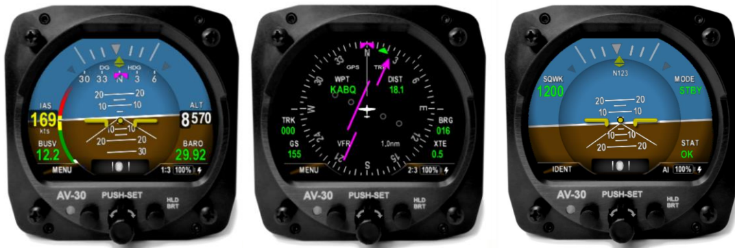
Figure 1 – AV-30-C Multi Mode AI/DG/Transponder – Basic Display
