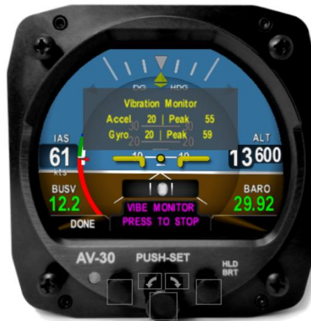
Figure 27 - Vibe Monitor Operation
