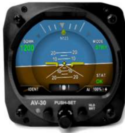
Figure 26 - Reversionary Attitude Indicator
