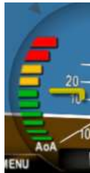
Figure 18 - AI Mode, AoA Indication
