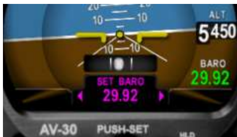
Figure 6 - Push-Set Example – SET BARO
