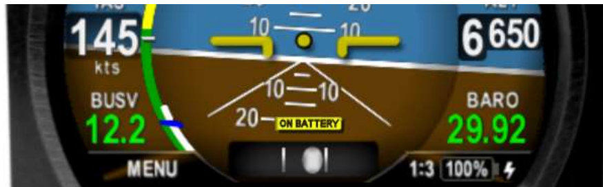
Figure 31 - On Battery Operation
