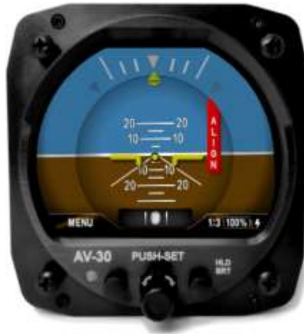
Figure 13 - AI Mode, Attitude Indicator
