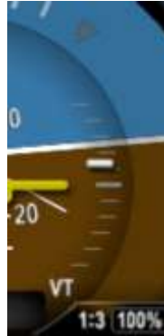
Figure 20 - AI Mode, Vertical Trend Indication
