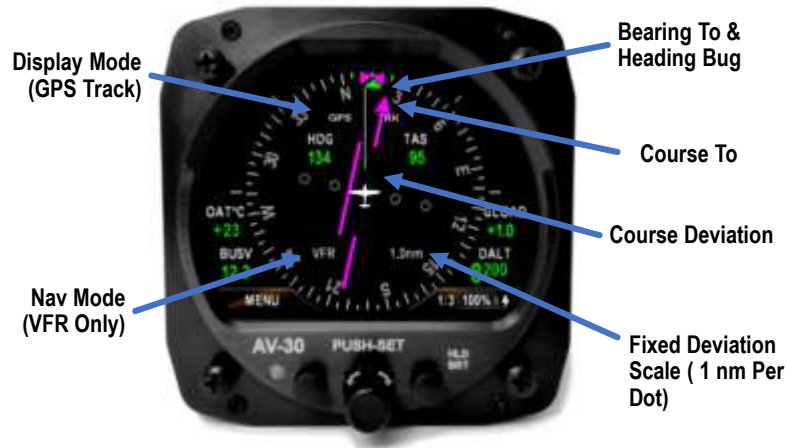
Figure 24 – GPS HSI Mode
