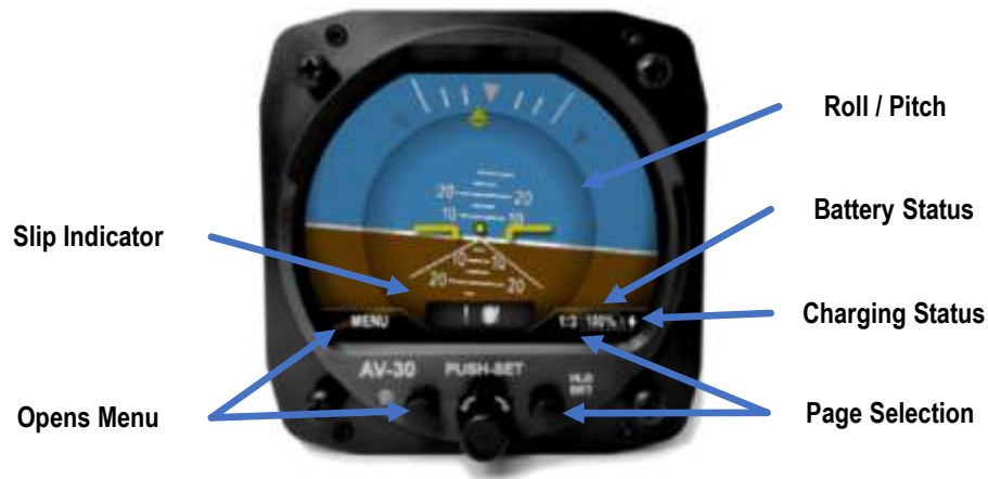
Figure 10 – Basic AI Mode User Interface
