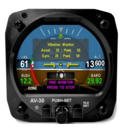
Record the data on the screen to share with uAvionix Support. Push and release the center knob again to stop monitoring vibration and return to the Installation Menu.
