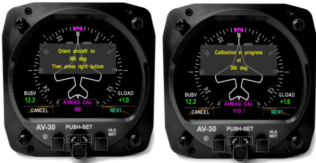
Figure 37 – AVMAG CAL In-Progress
