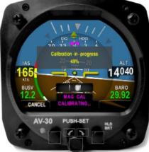
3. Fly for 10 minutes. Four, 360-degree standard rate turns will need to be completed. Each turn will represent 25% of the total.
