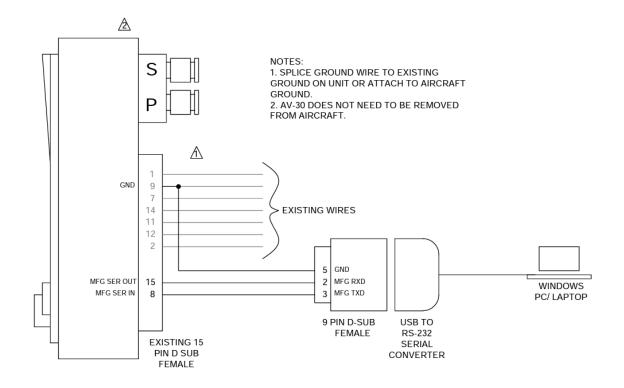
Note: AV-Link must not be installed if performing an update using the PC serial update procedure.
