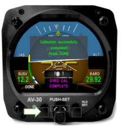
AV-30 will indicate "Calibration successfully completed Press DONE".
