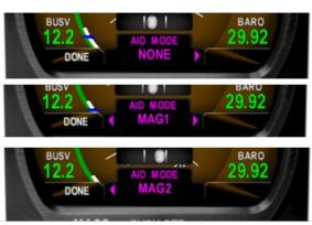
The factory setting for non-magnetometer equipped units is NONE, and the factory setting for magnetometer equipped units is MAG1. Leave the AID Mode set to the default, unless otherwise direct by uAvionix Support.
