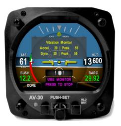
Record the data on the screen to share with uAvionix Support. Push the center button again to stop monitoring vibration and return to the Installation Menu.
