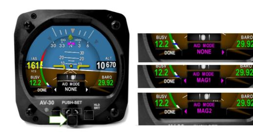
The factory setting for non-magnetometer equipped units is NONE, and the factory setting for magnetometer equipped units is MAG1. Leave the AID Mode set to the default, unless otherwise direct by uAvionix Support.
