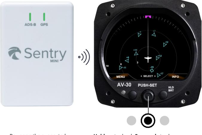
Power on the supported ADS-B Receiver **Hold** center knob **3 seconds** to change screens. Traffic Display is the third screen.
