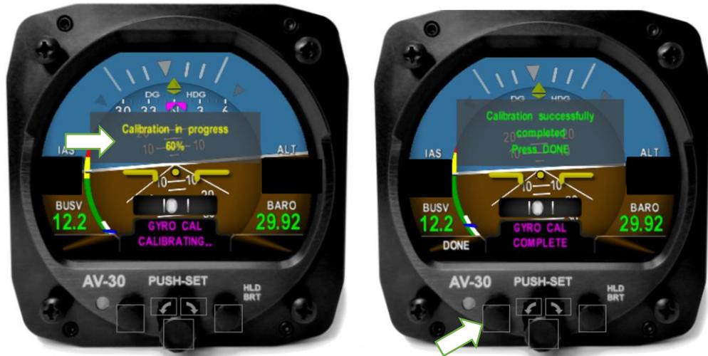
Figure 43 - Gyro Calibration Procedure
