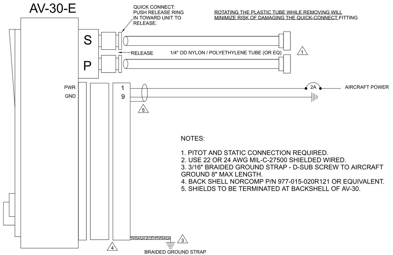
Figure 10 - Wiring Diagram – Required Connections
