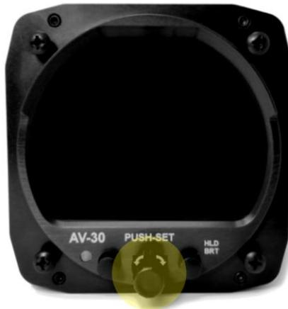
*Figure 35 – Installation Menu Access*
