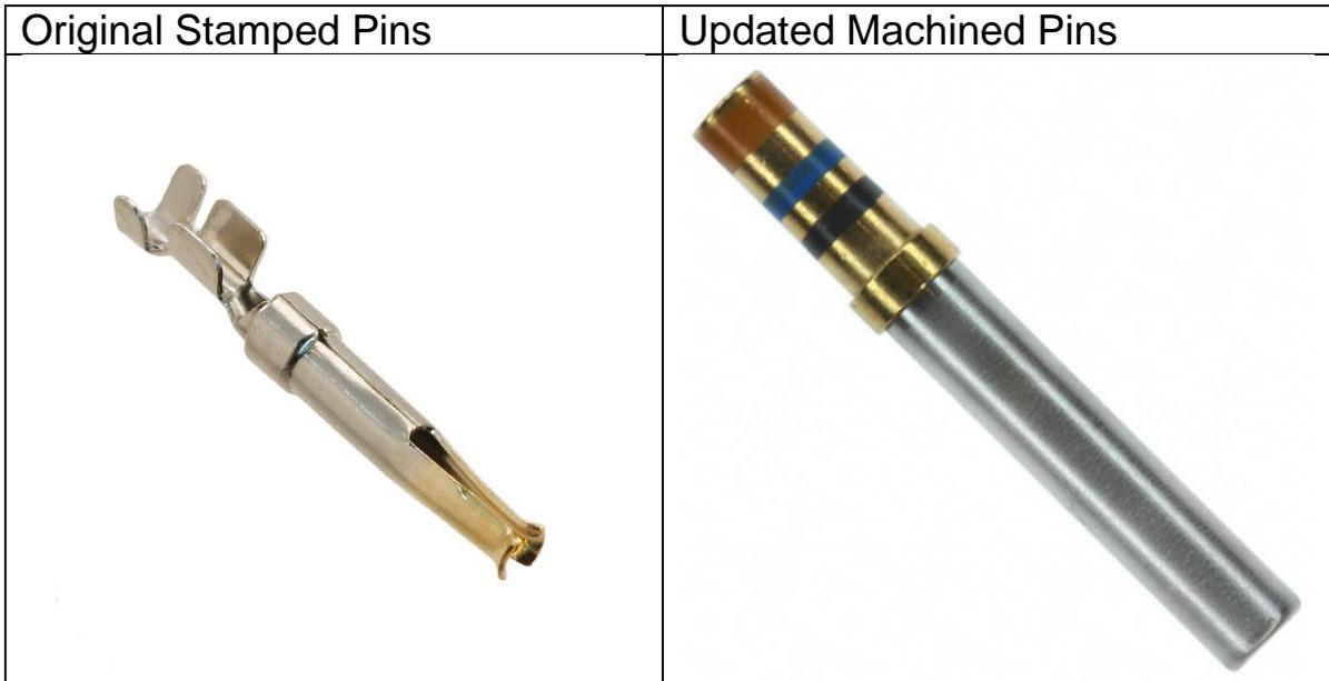
If your kit includes machined pins, a Daniels AFM8 crimp tool using a K13-1 positioner or equivalent M22520/2-01 tool should be used. If your installation kit includes the original stamped pins, a NorComp 180-701-170-000 hand crimper or equivalent should be used.
