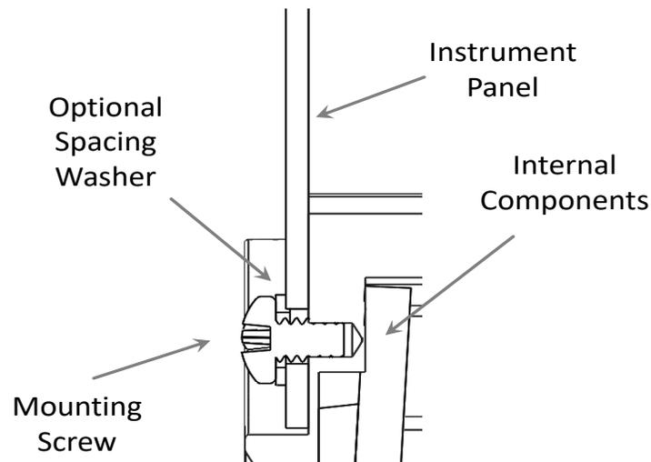
*Figure 6 – Mounting Screw Depth Limits*
