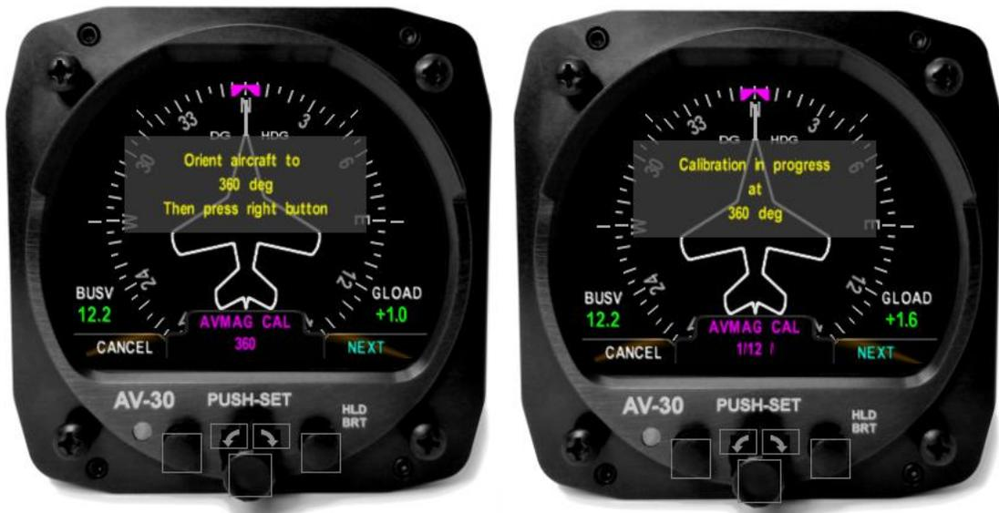
Figure 49 – AVMAG CAL In-Progress
