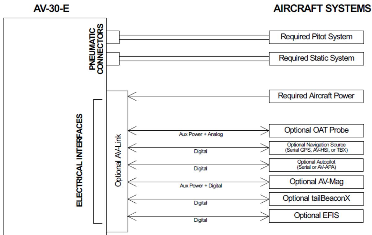
Figure 4 - AV-30 Aircraft Systems Interfaces – DG Mode
