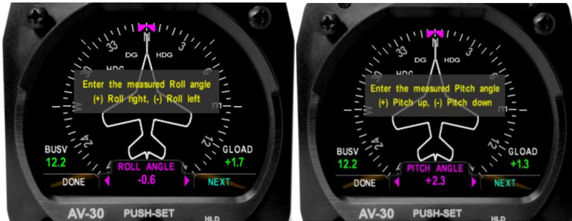
Once these values are committed, the AV-30 will calculate the differences in mounting angles for use in the heading solution. Once entered, changing these values without remeasurement of the AV-Mag angles will invalidate the installation calculation.
