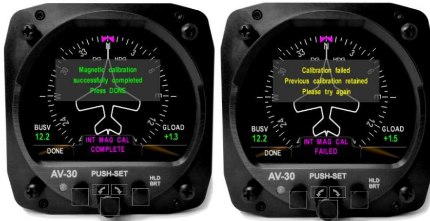
Figure 46 - INT MAG CAL Success and Failure Screens
