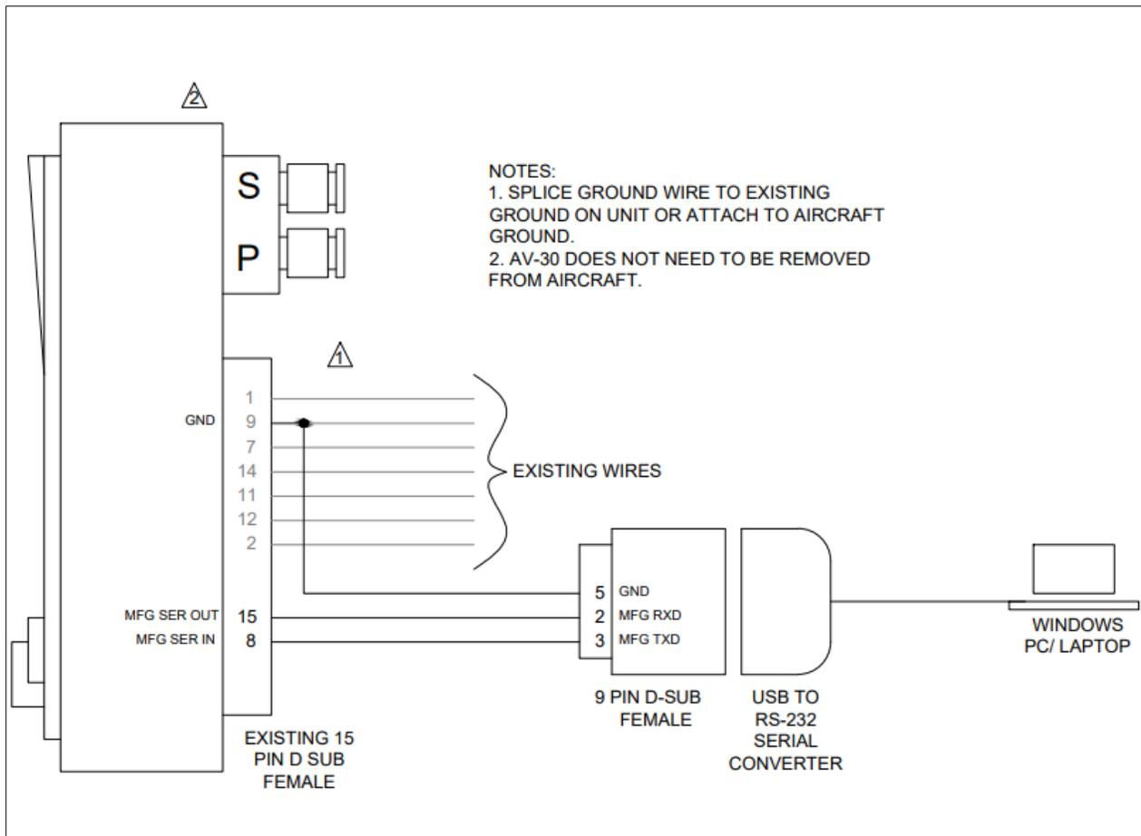
Figure 56 - Field Update Interface Diagram
