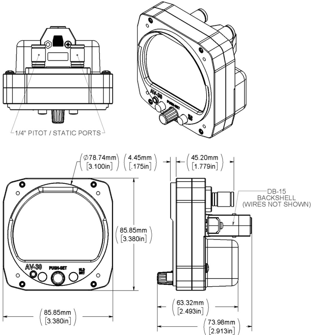
Figure 5 – Mechanical Drawing
