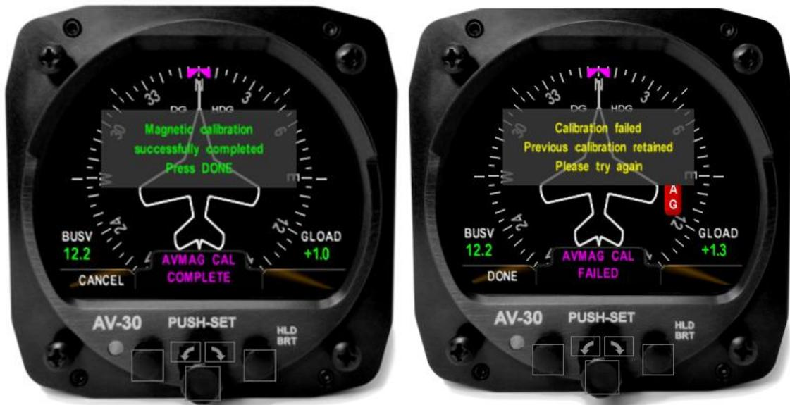
Figure 51 – AVMAG CAL Success and Failure Screens
