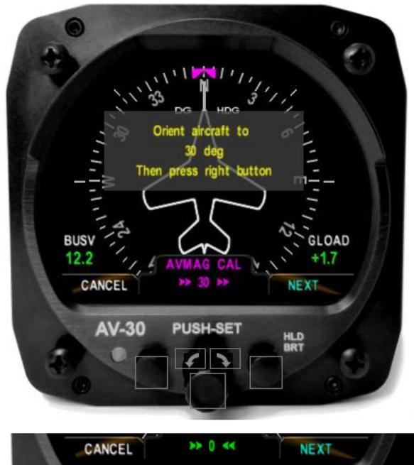
Figure 50 – AVMAG CAL Orientation Guide
