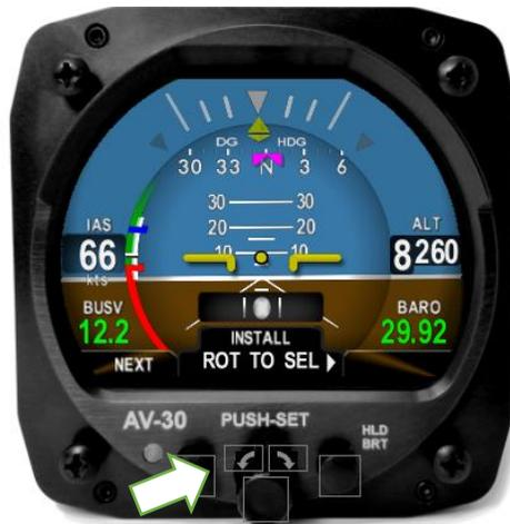
Figure 41 - Install Mode Selection
