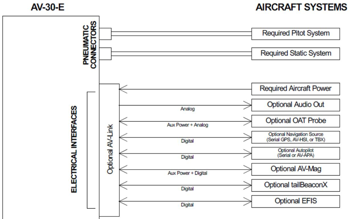
Figure 3 – AV-30 Aircraft Systems Interfaces – AI Mode
