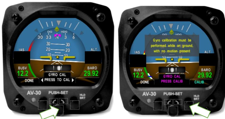
Figure 42 - Gyro Calibration Selection
