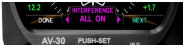
The deviation value indicates the magnitude and direction of the magnetic reading with respect to the Earth's magnetic field. A relatively small deviation near zero indicates little or no magnetic field interference, while a larger negative or positive deviation indicates the AV-Mag is sensing magnetic fields in addition to the Earth's.
