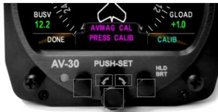
Figure 48 – AVMAG Calibration Entry
