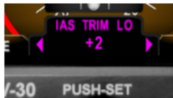
Now increase the airspeed on the air data test set to a value at least 70 knots higher than the airspeed used to set the LO trim point. Using your aircraft's high-speed cruise airspeed is recommended. Go to the IAS
