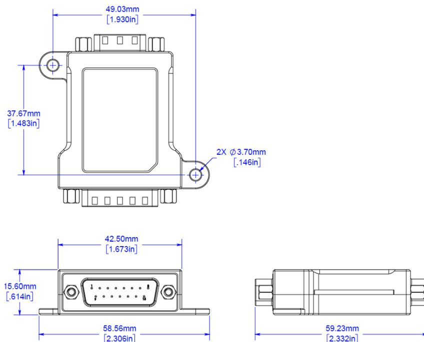
Figure 28 - AV-HSI Mechanical Drawing
