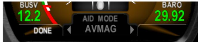
Enter the AV-30 installation menu again and navigate to the AV-Mag installation menu (AVMAG INSTL). Push the center rotary knob, then press the right button to begin the installation process. If AV-Mag is not properly connected, the version will indicate "Not detected".
