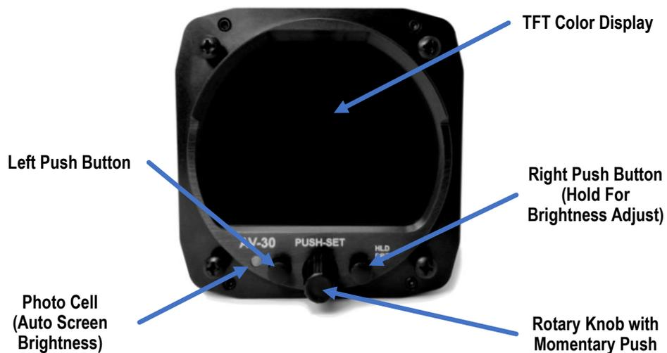
Figure 34 – Common User Interface Components
