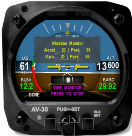
Figure 61 – Vibe Monitor Operation
