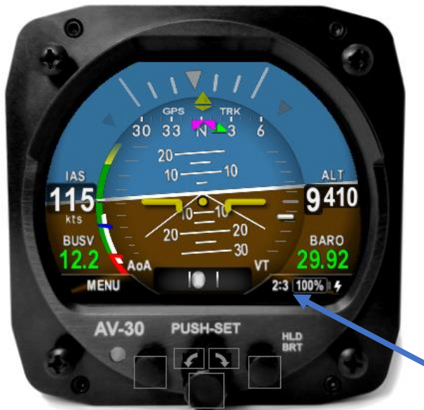
Figure 8 – Screen 2 of 3 showing GPS Ground Track, AoA, and Vertical Trend
