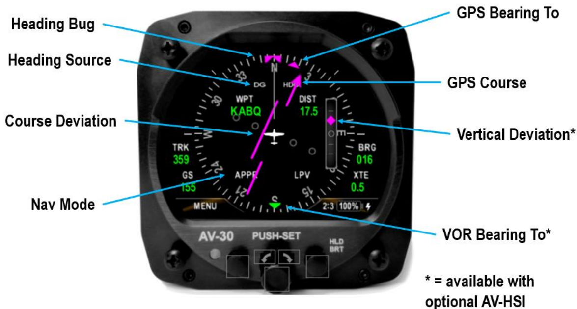
Figure 33 – Non-Slaved DG HSI User Interface
