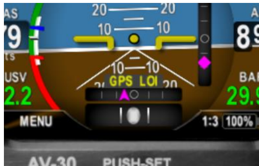
Figure 29 - AI Mode, GPS LOI Indication
