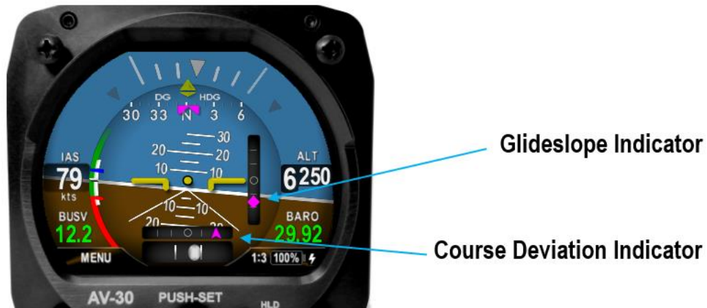
Figure 27 - AI Mode, Course Deviation and Glideslope Indication
