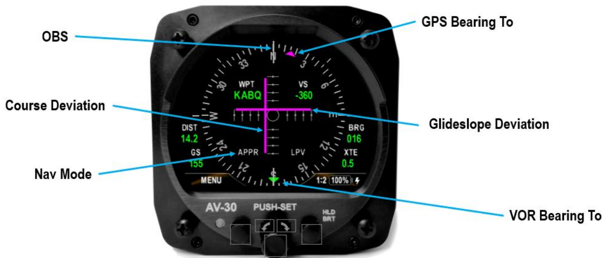
Figure 46 – CDI Mode with GPS Guidance
