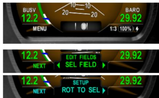
Figure 58 – Setup Menu Access
