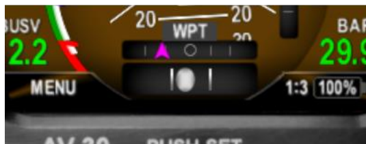
Figure 30 - AI Mode, Waypoint Indication
