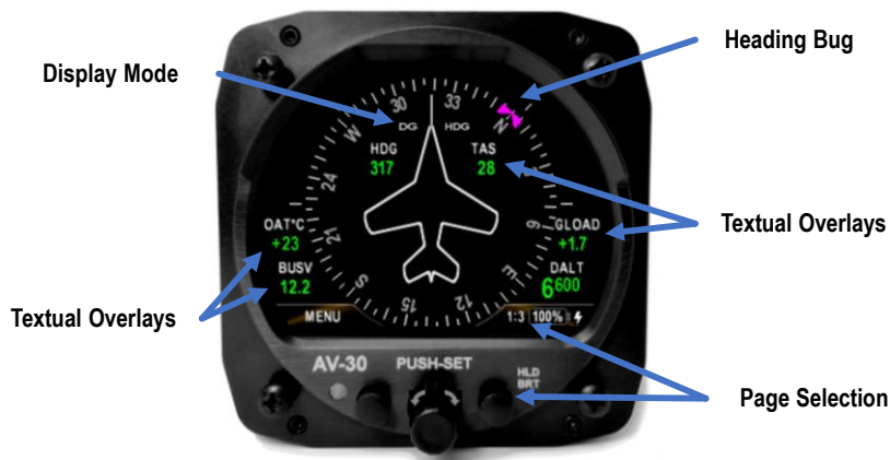
Figure 32 – Basic DG Rose Mode User Interface
