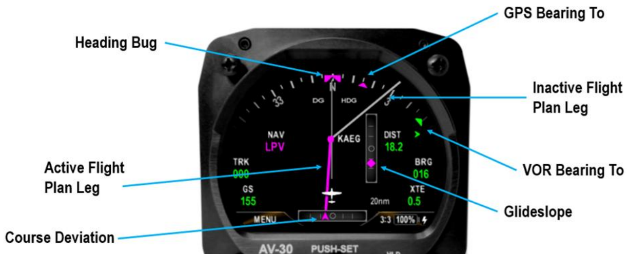
Figure 38 – Arc Mode with Course Deviation and Glideslope
