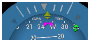
Figure 21 – AI Mode, Direction Indication, Bearing To Off-Screen
