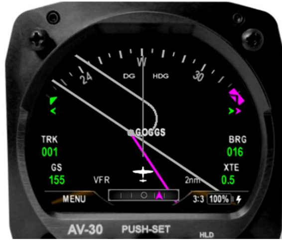
Figure 39 – Arc Mode with Holding Pattern
