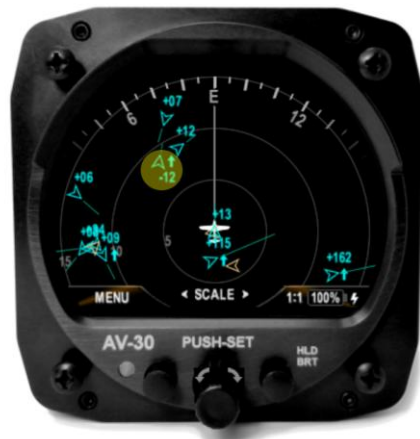
Figure 45 – Traffic Target Relative Altitude
