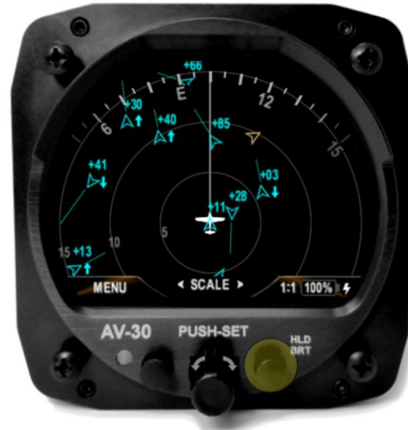
Figure 47 – Traffic Reversionary AI Activation
