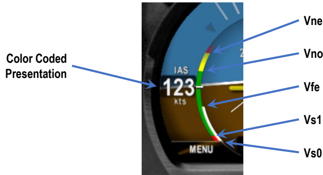
Figure 20 – AI Mode, V-Speed Limits
