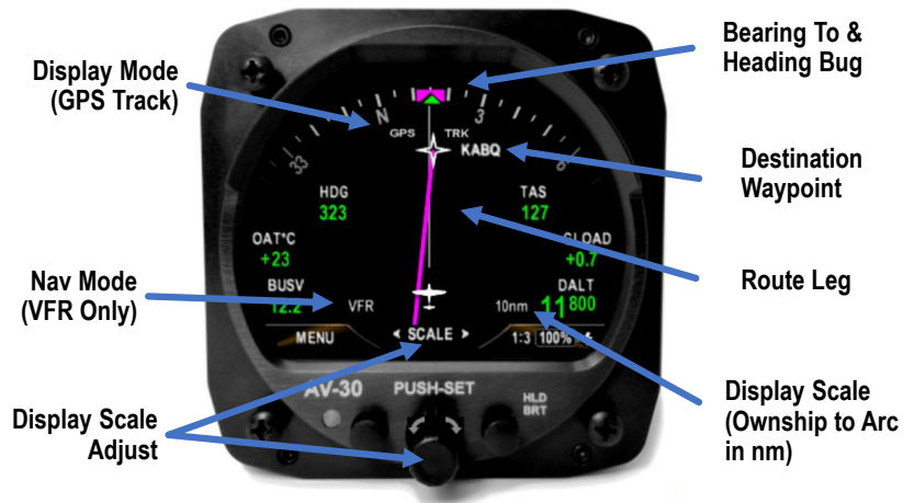
Figure 40 – Arc Mode without Course Deviation and Glideslope
