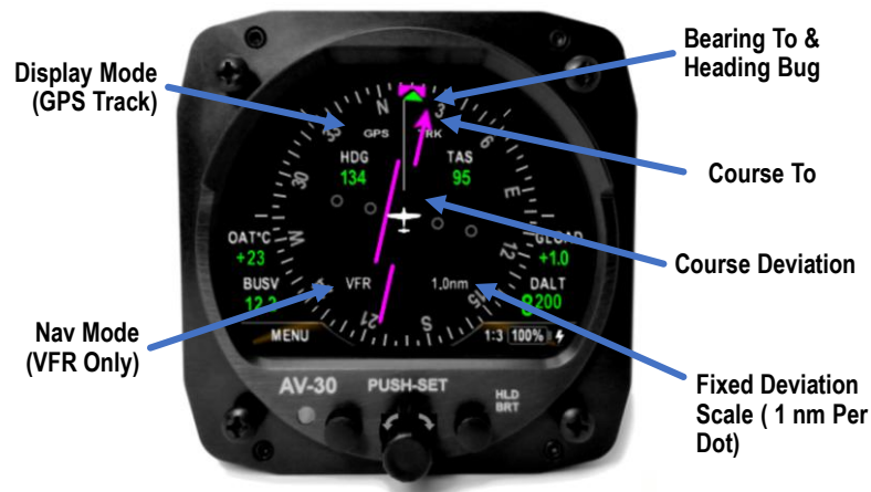
Figure 37 – GPS-Slaved HSI Mode with VFR GPS
