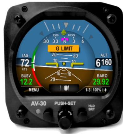
Figure 57 – Example of Alert Annunciator on Screen
