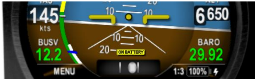
Figure 59 – On Battery Operation
