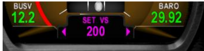
Figure 67 – Selected Vertical Speed entry
