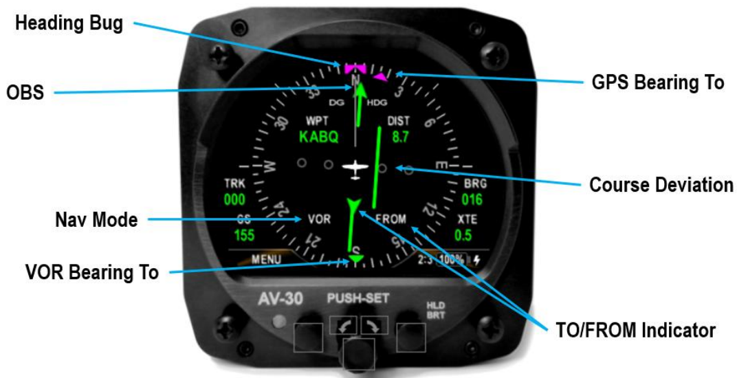
Figure 36 – Non-Slaved DG HSI User Interface with VOR Guidance
