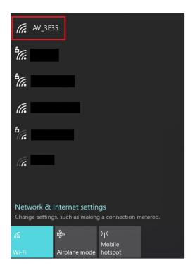
2. Connect a PC to the AV-Link-E Wi-Fi Network. This will be displayed as AV-### where #### will be 4 random characters ranging from 0-8 and A-F.
