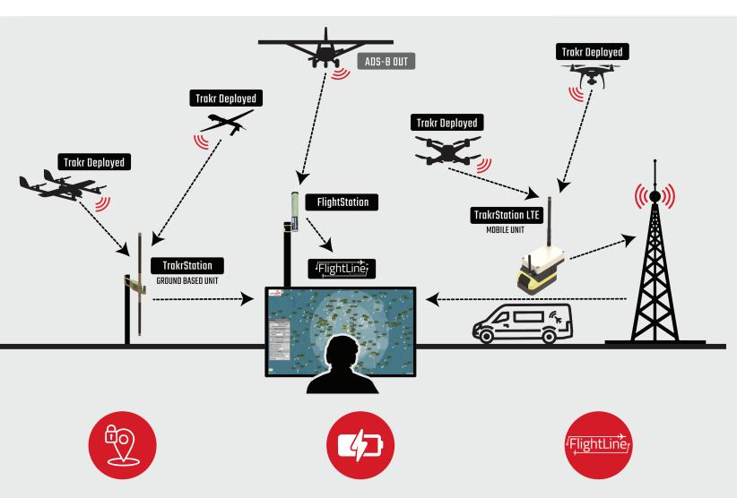
TrakrStations securely receive position data and push it to the cloud without exposing your fleet's flight details. This data is then visualized in the FlightLine situational awareness app, giving operators a real-time view of all Trakr-equipped drones in the mission area.
