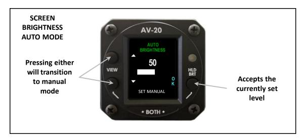
When in manual mode, pressing the up or down arrows will adjust the screen brightness. Pressing the right button will accept the value. Pressing ●BOTH● will revert to auto mode.
