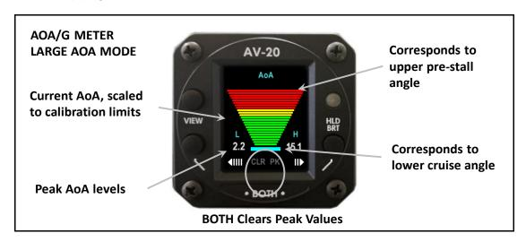
During power-on stabilization, the cyan lower bar will blink, indicating that no valid AoA can be determined. This applies to all color-coded AoA indications provided on different pages.
