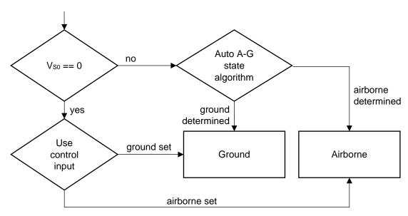
Airborne subsonic and supersonic state is automatically determined by ping200X.
