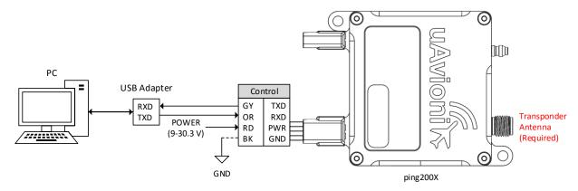
Set 'Conn Type' to 'Serial', 'Port' to the USB or serial port connected to the ping200X, 'App Baud' to '57600' and 'Protocol' to 'UCP'.
