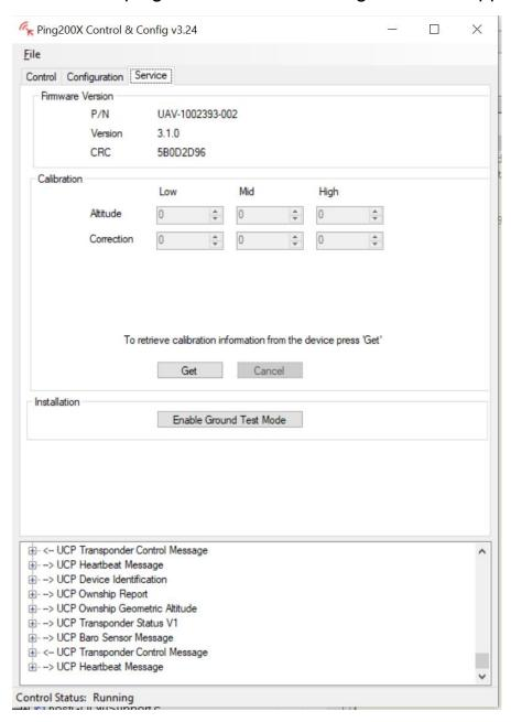
Confirm the displayed 'P/N' and 'Version' on the 'Firmware Version' section of the 'Service' tab is current per Service Bulletins listed at:
