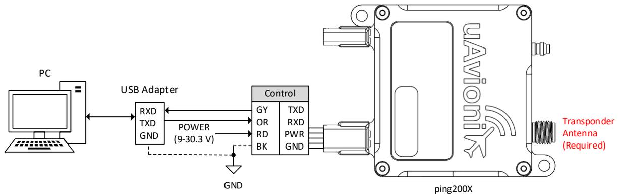
Set 'Conn Type' to 'Serial', 'Port' to the USB or serial port connected to the ping200X, 'App Baud' to '57600' and 'Protocol' to 'UCP'.
