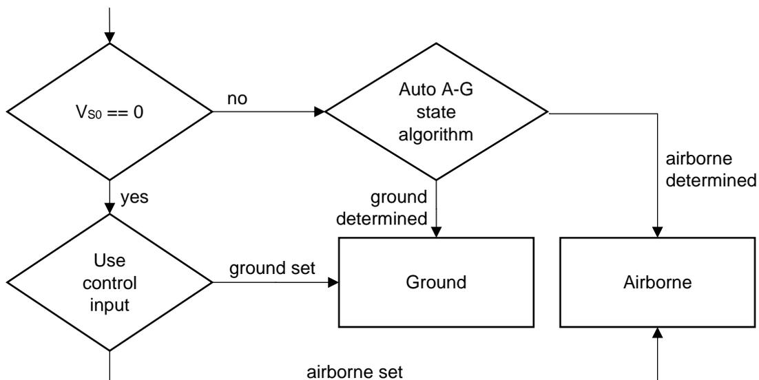
Airborne subsonic and supersonic state is automatically determined by ping200X.
