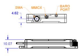
Whenever power is supplied to the transponder, a 500hm load must be provided to the SMA connection. You can use the supplied antenna or a commercially available 500hm load.
