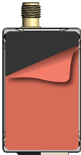
**Mount ping20S** to a suitable flat surface using the provided **double-sided mounting tape**. Affix mounting tape to ping20S and attach the transponder to the aircraft.
