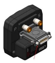
Reattach the original AV-30 Backshell Connector. Using a flat screwdriver, tighten the two [2] screws to 5in\*lbs max. Do Not Overtighten!
