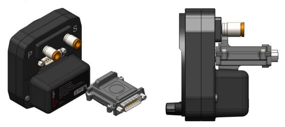
Using a 3/16" nut driver, tighten the two [2] Jack Screws to 5in\*lbs max. Do Not Overtighten!
