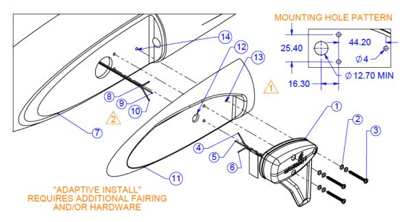
skyBeacon is mounted with three 6-32-inch screws to the existing holes and nut plates in the end of the wing, with the wingtip adapter sitting between the wing and skyBeacon.
