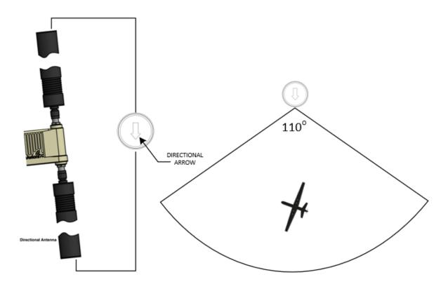
Figure 3 Directional Antenna Orientation
