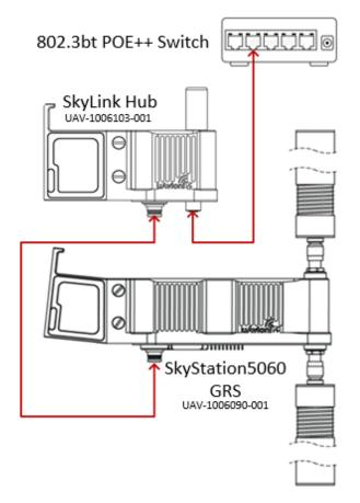
Figure 5 – SkyStation5060 GRS Connections
