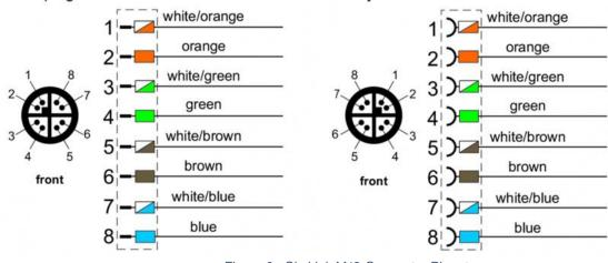
Figure 6 - SkyLink M12 Connector Pinout
