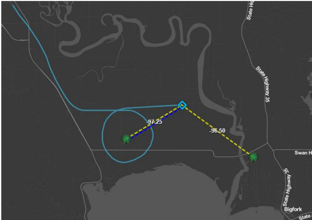
When a GRS receives messages from the aircraft, a binding line between the two devices will appear. These lines will be either green, yellow, or red in color based on the signal strength. A blue binding line indicates that the aircraft is linked to that GRS. When the device roams, the blue line will switch to the next linked GRS.
